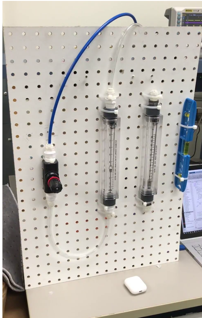
Figure 3.12: Flow adjustment valve and meter
