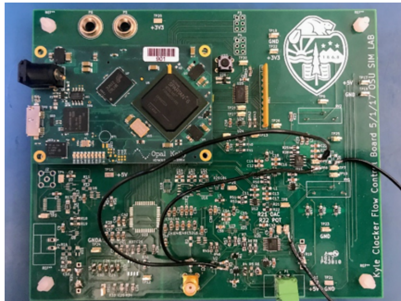
Figure 3.4: Photograph of the completed test PCB used to test the dual-slope control algorithm using the single-element thermal flow sensor.
