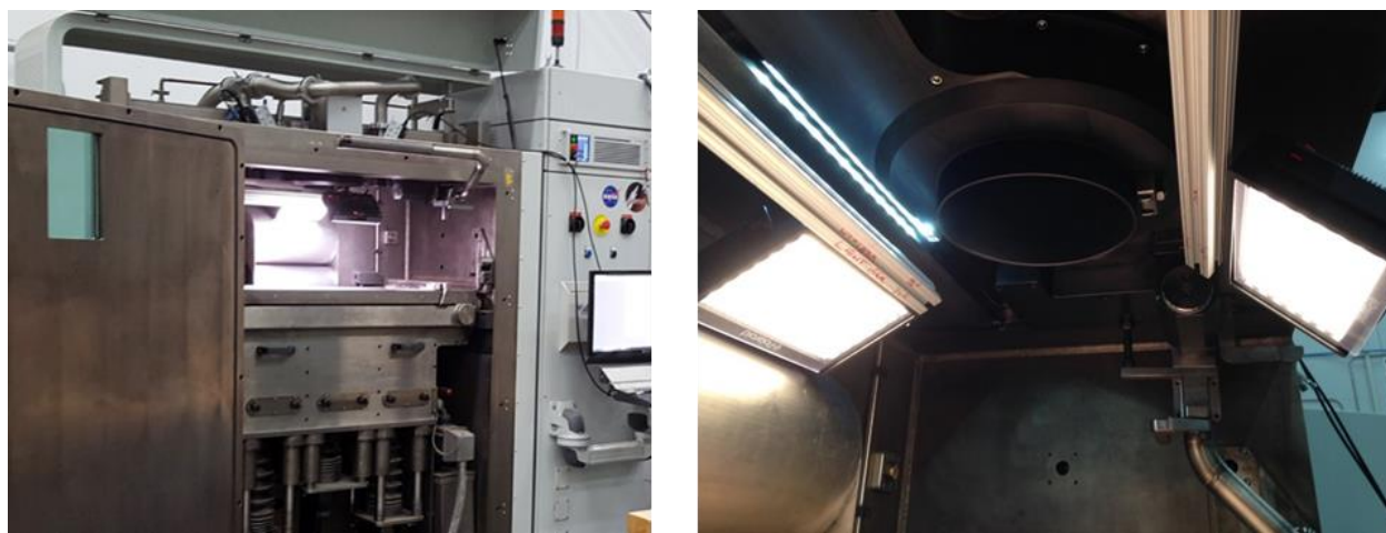
Figure 2.2: Polarized LED light panels were employed in tandem with adjustable lens polarization filters to improve the contrast of metal powder surfaces and suppress reflections that inhibited the stereo correlation process.
