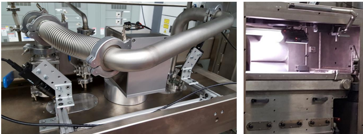
Figure 3.3: Actual vision system implementation with custom viewing windows (left) and polarized internal chamber lighting (right).
