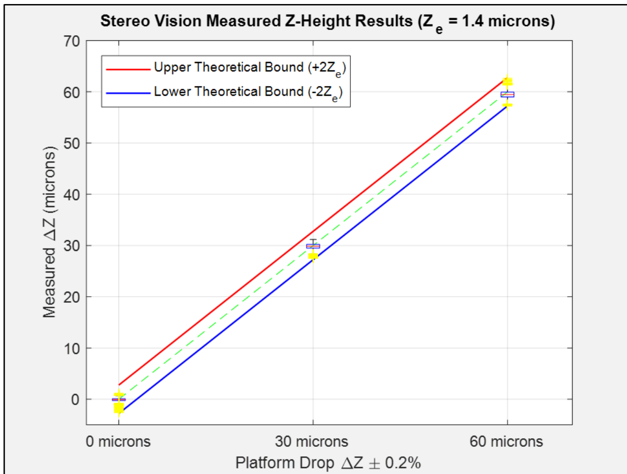
Figure 2.8: Plot of experimental \Delta Z data with corresponding maximum and minimum bounds provided by the theory ( \epsilon = 0.073 pixel, \min(\Delta D) = 0.063 pixel, B = 687 mm, Z = 600 mm). The 8,892 measurements made at each platform position are displayed as boxplots for convenience (yellow “+” indicates outliers).
