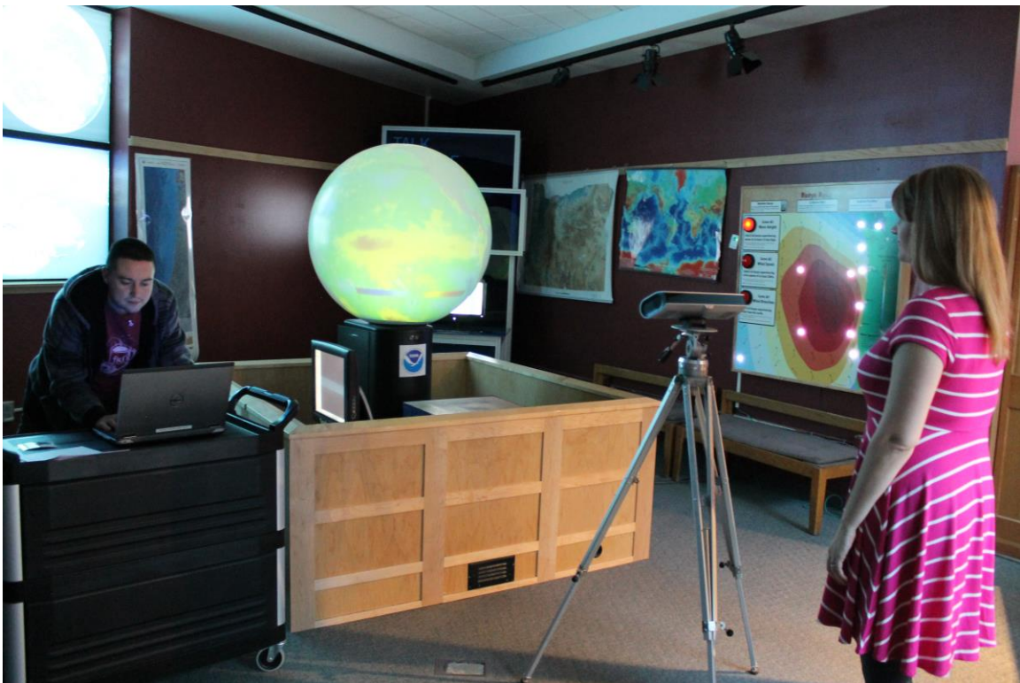
Figure 2. In situ Eye-tracking setup. The participant, right, stands in front of the eye-tracker on a tripod in front of the exhibit. The researcher, left, controls the eye-tracker via computer and also presents the stimulus image on the globe using the touch screen monitor at the lower-left of the globe. Here, the stimulus image is the unscaffolded version of the Sea Surface Temperature Anomaly visualization, with color bar visible on the globe at the bottom of the visualization.
