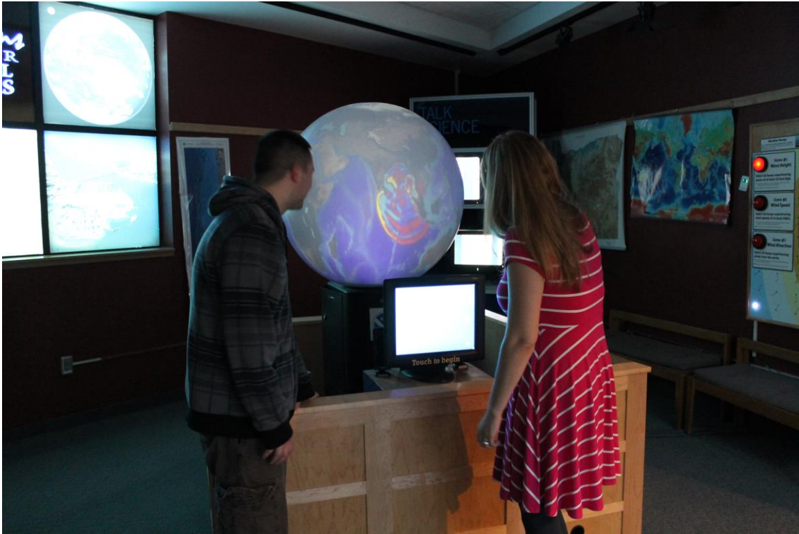
Figure 1. Example of Spherical Display System exhibit. Visitors view the Magic Planet™ 3-foot diameter spherical display system with interactive touch-screen kiosk.
