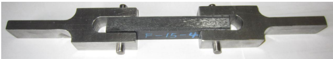
Figure 21 15° flange specimen in clevis fixture
