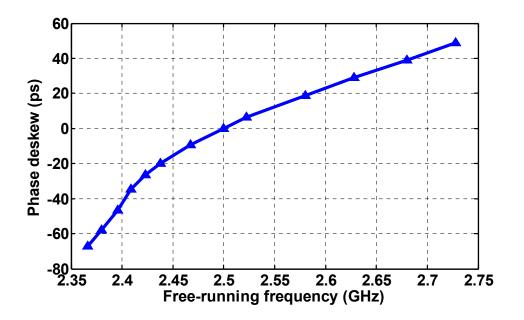
Figure 4.14. Deskewing of ILRO by tuning free-running frequency.
