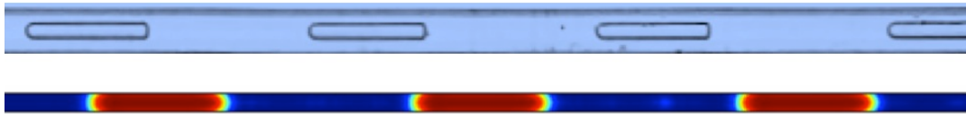
Figure 4.8 Experimental results (upper) and simulation results (lower) for Jatropha oil/N 2 . Red = Gas phase, Blue = Liquid phase.
