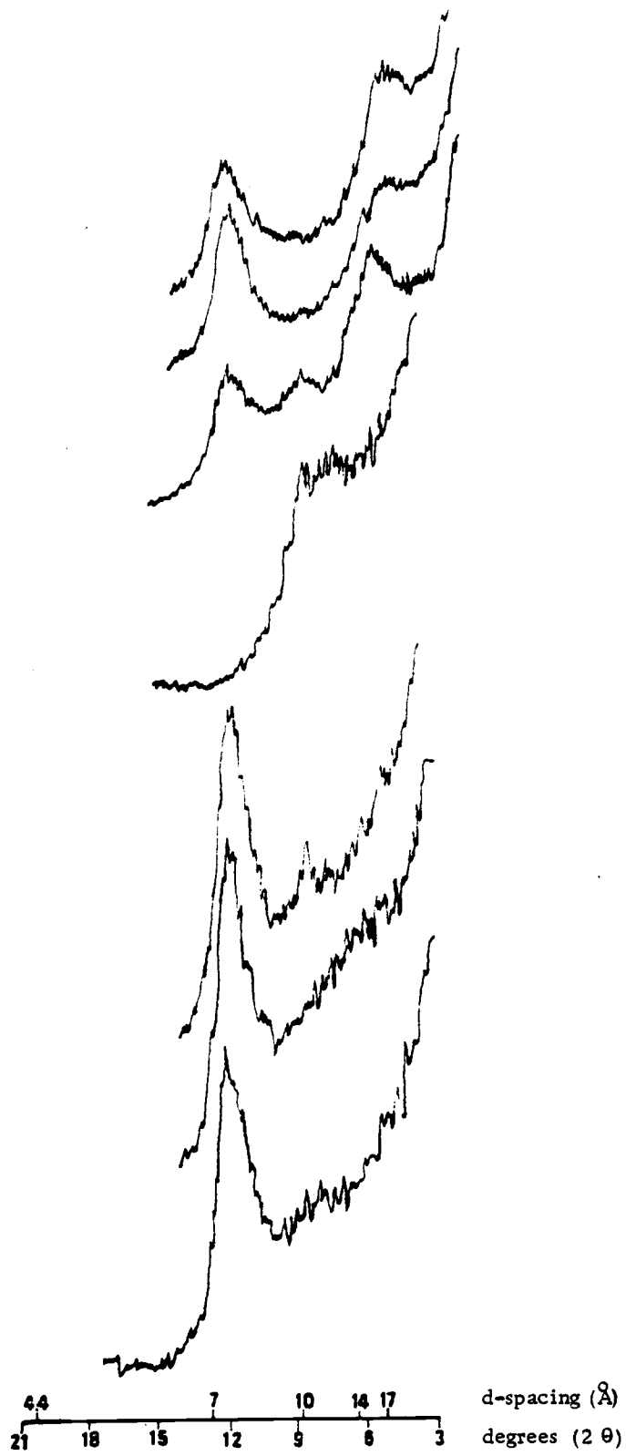
Typical XRD pattern of slump-earthflow sites. Cu K \alpha source, 35 kv, 25 ma.
