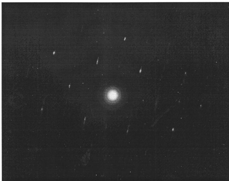
Figure A.3.1.4. The whiskers are crystalline which is shown by the spot pattern from electron diffraction. No spot pattern was observed for the bulk structure.
