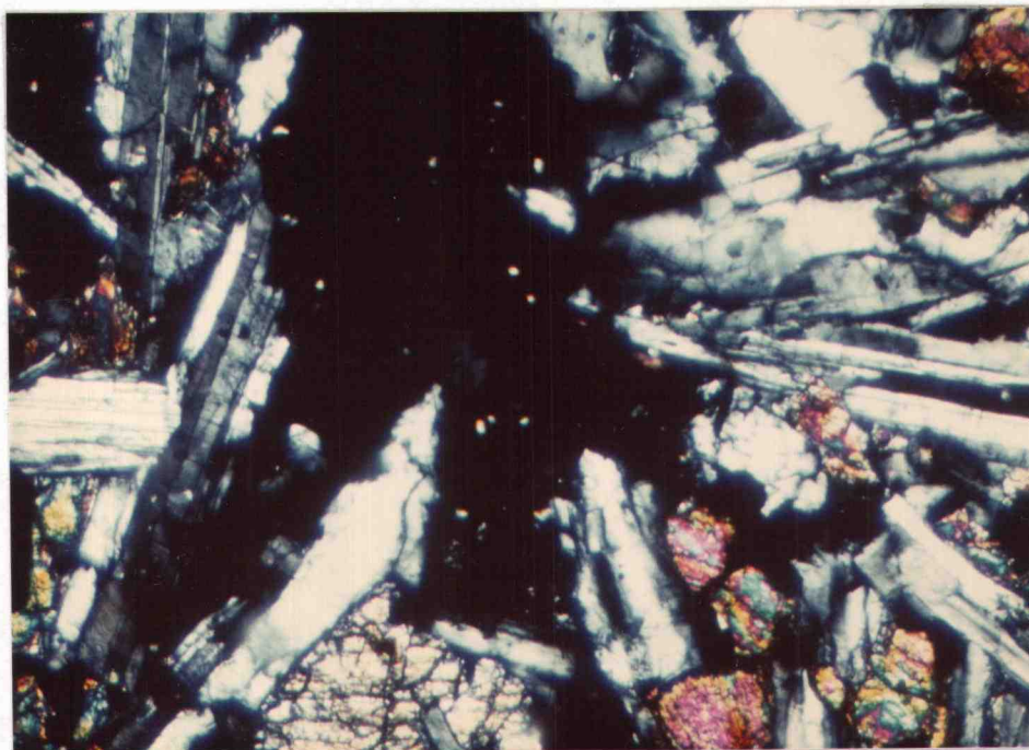
Figure 12. Laths of plagioclase showing diktytaxitic texture in Steens Basalt (X20, cross-polarized light).
