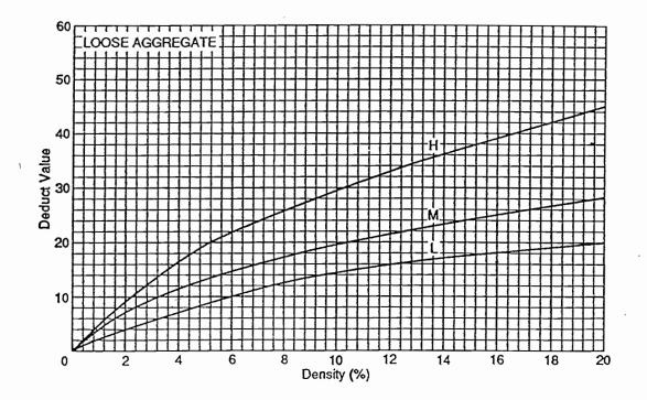
Figure 57. Loose Aggregate.
