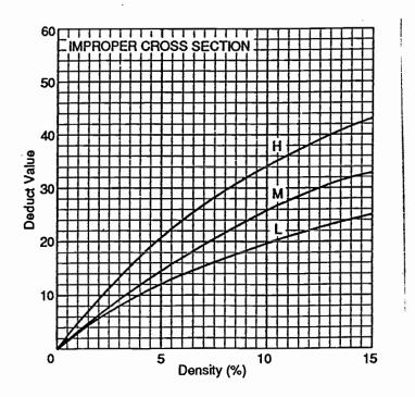
Figure 51. Improper Cross Section.
