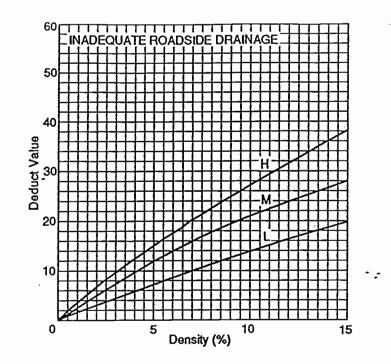
Figure 52. Inadequate Roadside Drainage.
