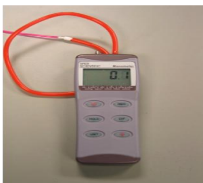
Figure B.5. Manometer
