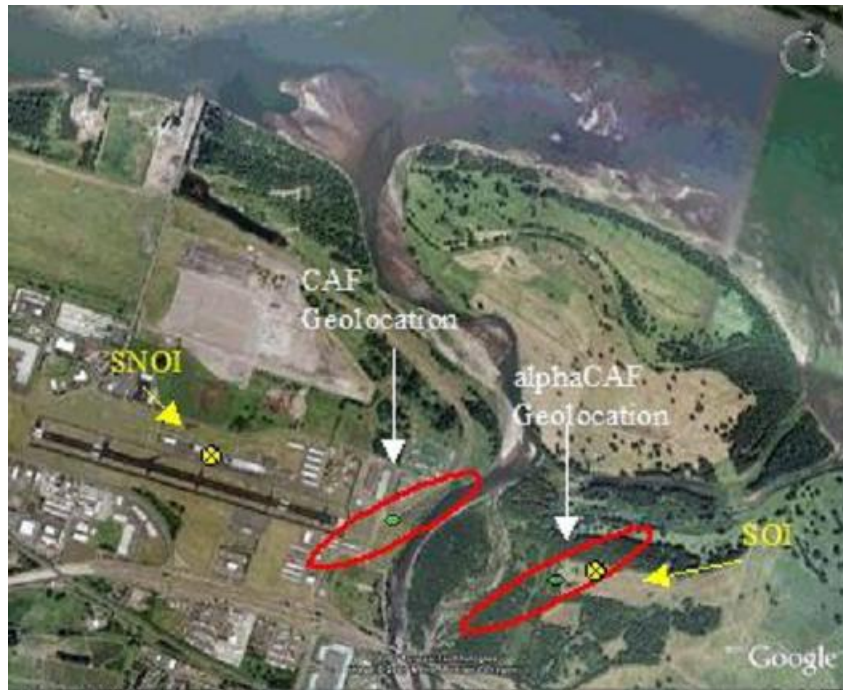
Figure 7.5: Simulated example of geolocation of a lost hiker in a co-channel signal environment using both the conventional CAF method and the new \alpha -CAF method. Computed location estimates are overlaid on an aerial photograph. The actual location of the SNOI emitter is at the airport. The hiker location is marked in the open space to the right of the airport. The computed geolocation results are overlaid on the photograph showing that the conventional CAF method produced biased TDOA and FDOA measurements and therefore an incorrect geolocation. The \alpha -CAF method produced good TDOA and FDOA estimates allowing the hiker to successfully be located.
