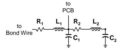
Figure 2.3: Model used to represent the parasitics of the package.
