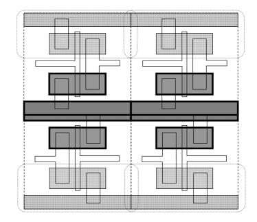
Figure 6.2: Example of defined substrate contacts for individual gates overlapping in the layout.
