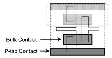
Figure 6.1: Substrate contacts defined for a single gate.
