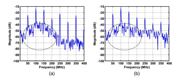
Figure 4.2: Comparison of frequency domain (a) measurements, and (b) simulations for the CBL PRNGs.
