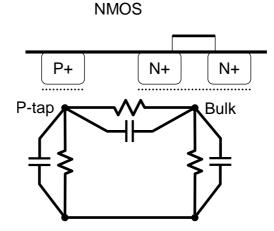
Figure 5.4: The substrate  $\pi$ -network incorporating higher frequency effects.
