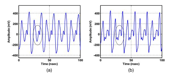
Figure 5.2: Comparison between (a) the complete simulation of the CBL PRNGs, and (b) the same simulation with coupling capacitances between interconnects removed.
