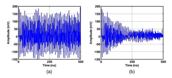
Figure 4.5: Comparison of a test setup with the NCL PRNGs with (a) constant Vth, and (b) varied Vth.
