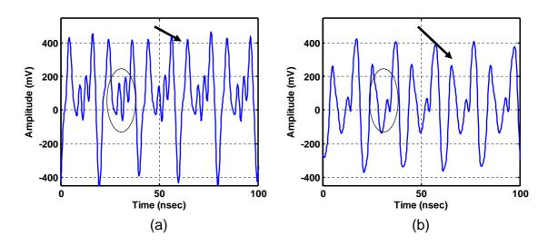
Figure 4.1: Comparison of time domain (a) measurements, and (b) simulations for the CBL PRNGs.
