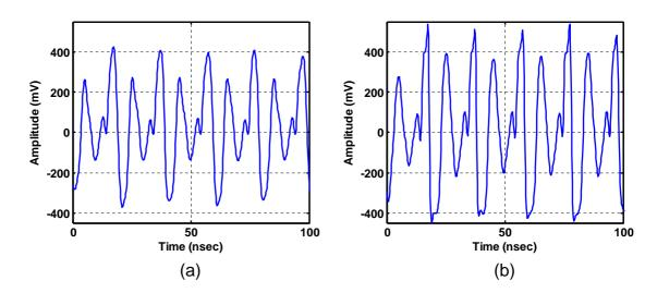
Figure 4.7: Comparison of time domain (a) transistor level simulations, and (b) DMM simulations for the CBL PRNGs.
