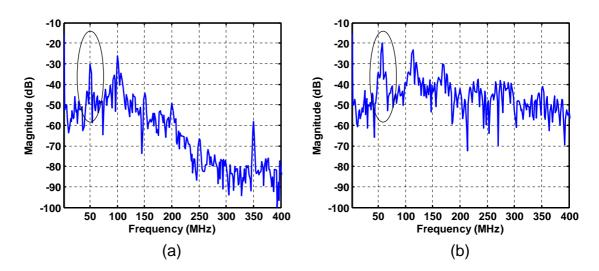
Figure 4.6: Comparison of frequency domain (a) measurements, and (b) simulations for the NCL PRNGs.
