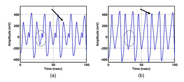
Figure 5.1: Comparison between (a) the complete simulation of the CBL PRNGs, and (b) the same simulation with the IO buffers' substrate network removed.
