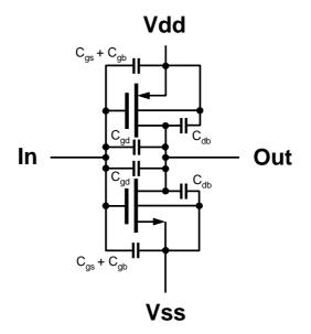
Figure 3.2: The parasitics of a simple inverter.
