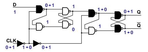
Figure 3.6: Internal logic branches switching when a D-type flip-flop changes states.
