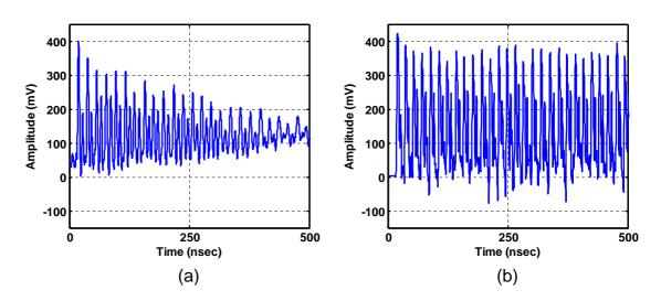
Figure 4.4: Expanded time scale comparison of (a) measurements, and (b) simulations for the NCL PRNGs.
