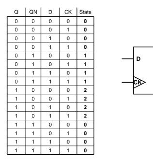
Figure A.2: Example of a state map for a simple D-type flip-flop.
