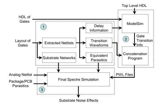
Figure 3.1: Flow chart showing all the steps in the digital macro-modeling (DMM) method.
