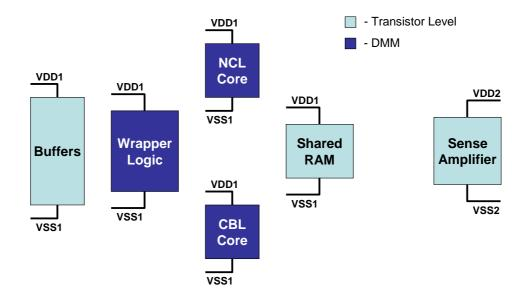
Figure 2.2: Block diagram showing the circuit setup for the simulation of the 8051 microprocessor cores.
