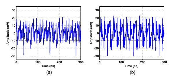
Figure 4.9: Comparison of time domain (a) measurements, and (b) DMM simulations for the CBL 8051 microprocessor core.
