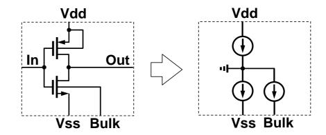
Figure 1.1: Model previously used to represent the digital gates.
