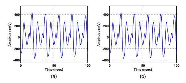
Figure 5.3: Comparison between (a) the complete simulation of the CBL PRNGs, and (b) the same simulation with the pad capacitances to substrate removed.
