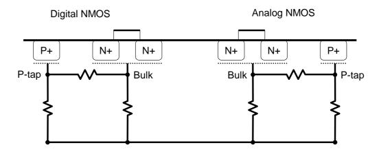
Figure 2.5: Model used to represent the substrate.
