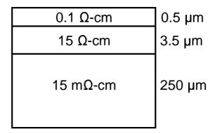
Figure 2.4: Approximated 3-layer profile for the TSMC  $0.25\mu$ m heavily doped substrate.
