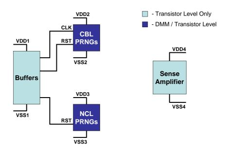
Figure 2.1: Block diagram showing the circuit setup for the simulation of the PRNG blocks.
