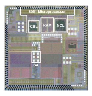
Figure 1.3: Die photo for Eris test chip.
