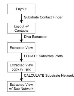
Figure B.6: Flow chart describing the steps to use Silencer! Extracted.
