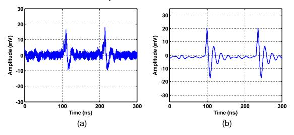
Figure 4.10: Comparison of time domain (a) measurements, and (b) DMM simulations for the NCL 8051 microprocessor core.
