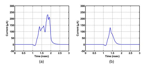
Figure 3.4: Supply current of a flip-flop for a given input pattern when the output (a) changes state, and (b) remains the same.
