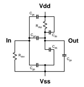
Figure 3.3: Equivalent parasitics of an inverter when the input is held low and the overlap capacitances are ignored.
