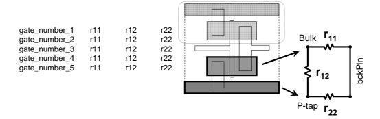
Figure A.3: Representation showing the way the resistive substrate model for each gate is saved.
