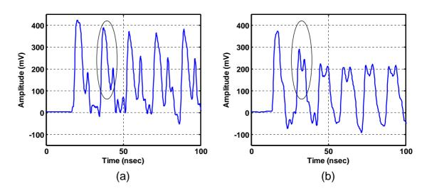
Figure 4.8: Comparison of time domain (a) transistor level simulations, and (b) DMM simulations for the NCL PRNGs.
