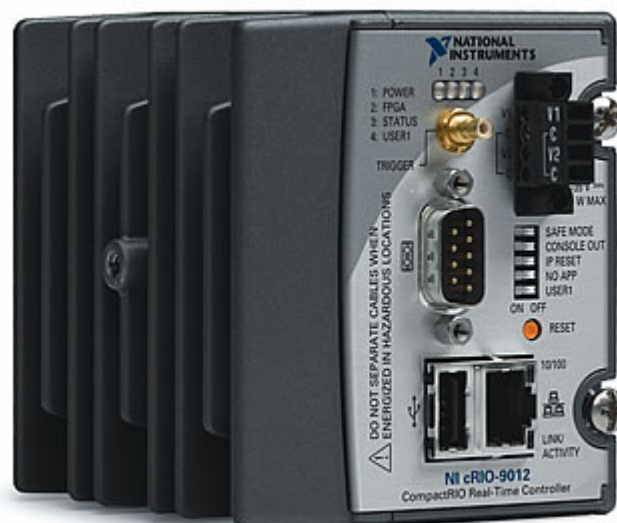
Figure 6.5 – cRIO Real-Time Controller [28].
