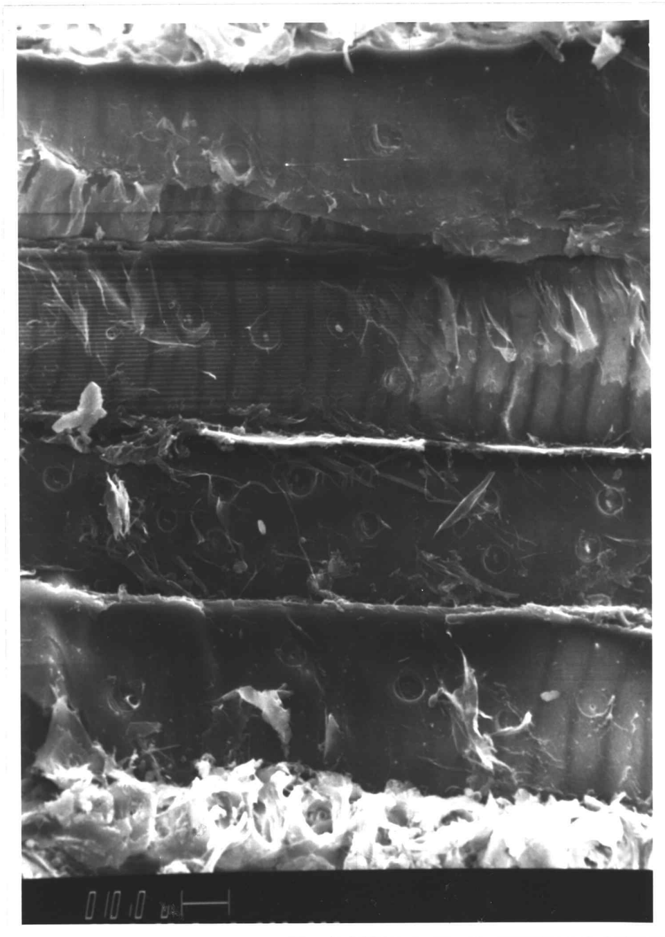
Figure II-2. SEM of wood samples from the study log. (B) Under- side of a surface scraping. Bar, 10 \mu .
