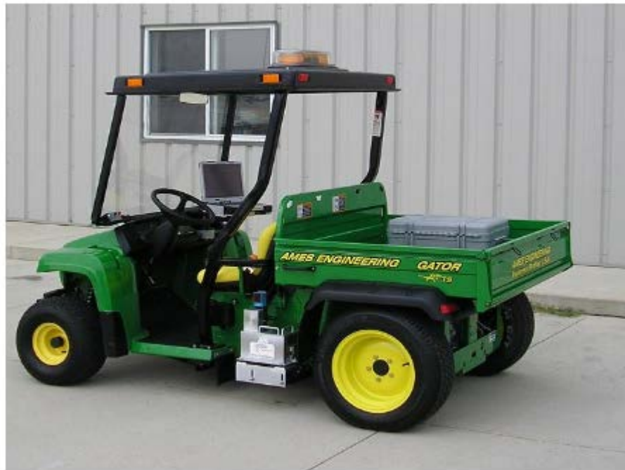
Figure 5.1: Example of a light weight inertial profiler (from Ames Engineering 2010)
