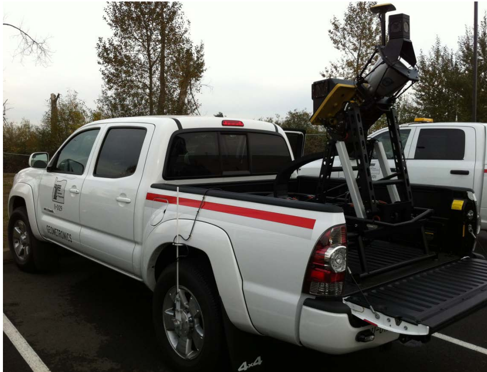
Figure 2.6: ODOT's mobile laser scanner
