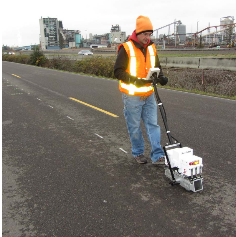
Figure 2.2: SurPRO inclinometer operated by ODOT
