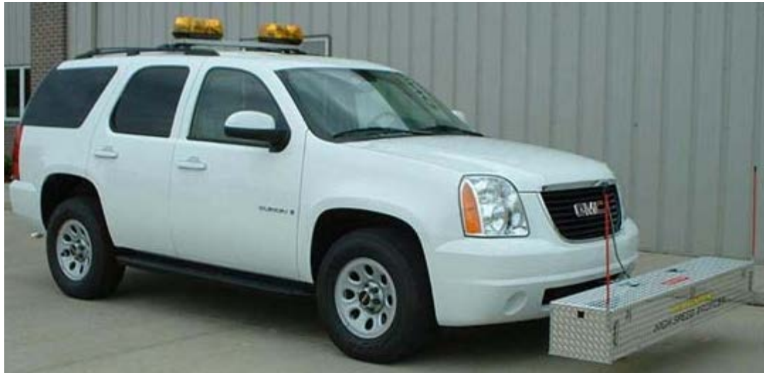
Figure 2.3: High speed inertial profiler (from Ames Engineering 2010)
