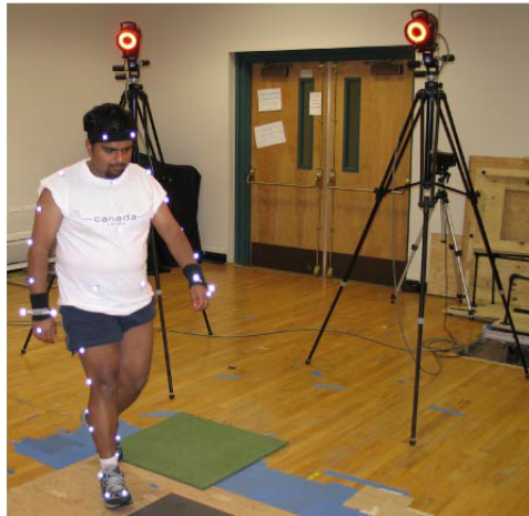
FIGURE 1.1. Impression of motion capture system. Highly reflective optical markers placed on subject are recorded by infrared cameras as he walks.
