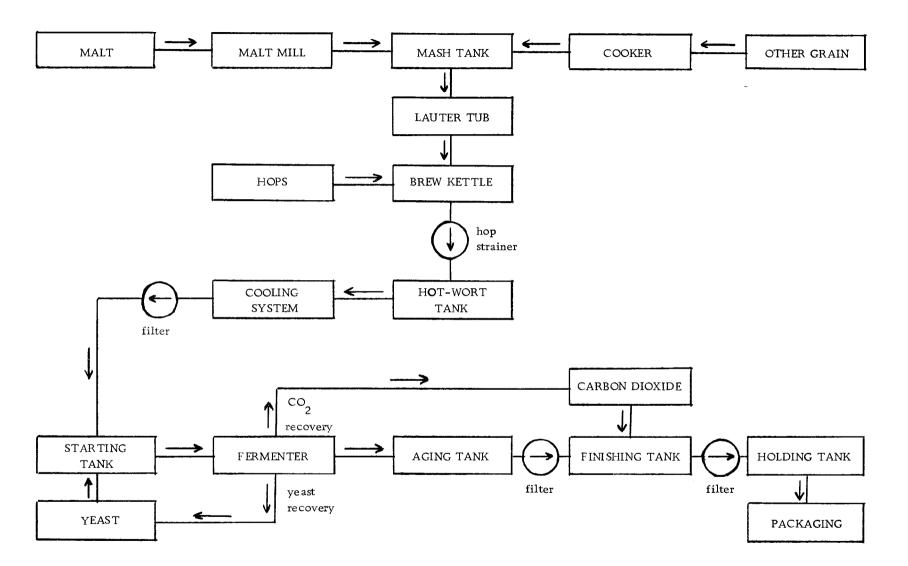
Figure 1. A typical brewery flow diagram.
