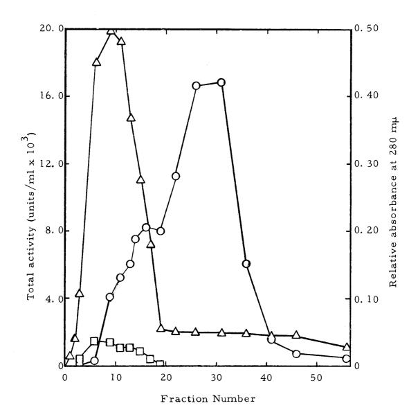
Figure 12. Sephadex elution pattern showing total activity of NADH oxidase (- $\Box$ -), total activity of diacetyl reductase (-O-), and relative absorbance (- $\Delta$ -) of each 1.35 ml fraction eluted from a 2.5 by 36.0 cm column of G-200 Sephadex.
