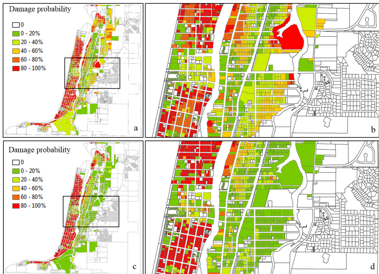
Fig. 3.8 Spatial distribution of probability of complete damage from 1,000-year event using two types of fragility curves. (a) S2013 model, (b) detail, (c) FEMA model, and (d) detail.
