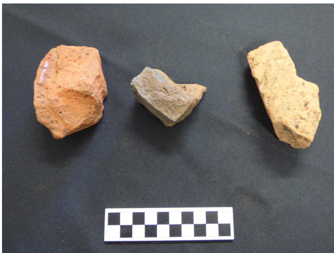
Figure 4.9 Fragments of brick showing variation in color found in the site caused by inconsistent kiln temperatures, common with temporary kilns
