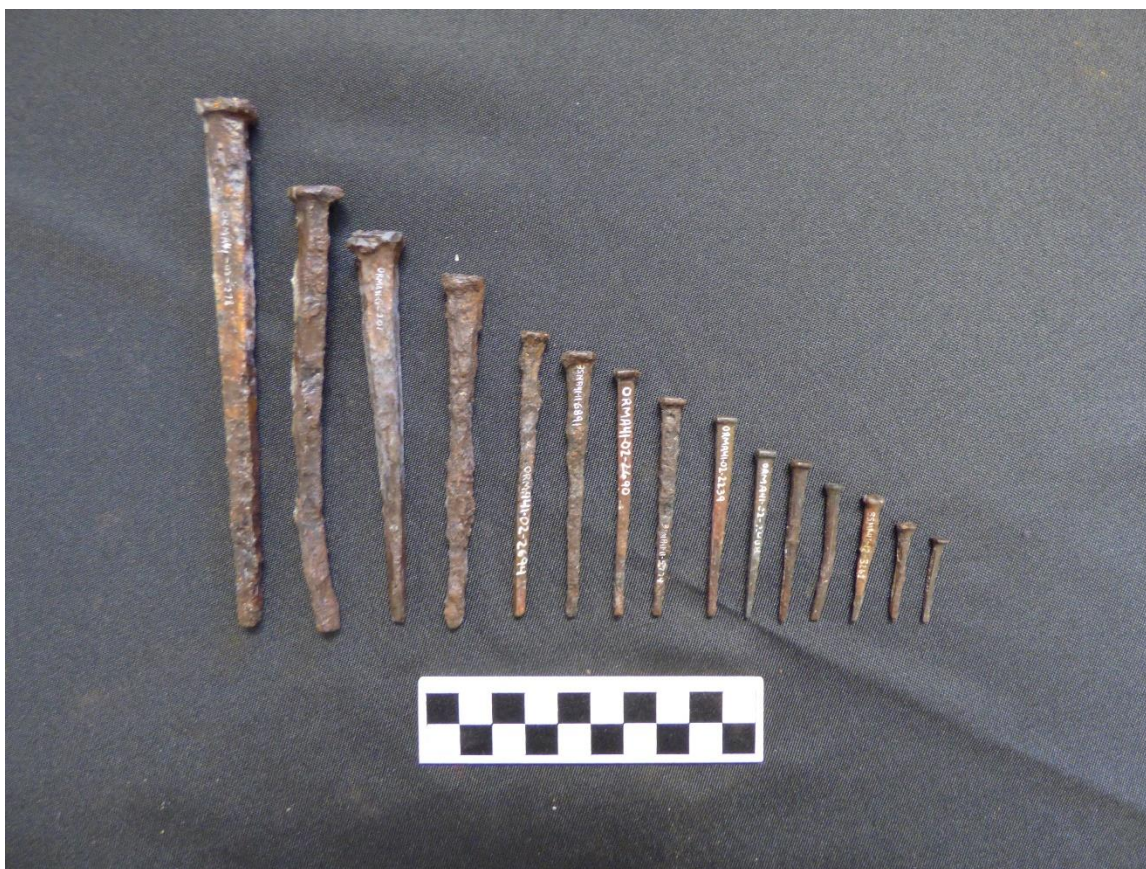
Figure 4.3 Machine cut square nails from site, left to right 60d, 40d, 30d, 20d, 16d, 12d, 10d, 9d, 8d, 7d, 6d, 5d, 4d, 3d, 2d
