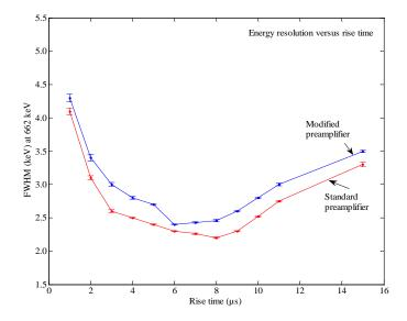
Figure 4.11 Energy resolution versus rise time in the trapezoidal filtering (flat top time was fixed at 0.8 µs).
