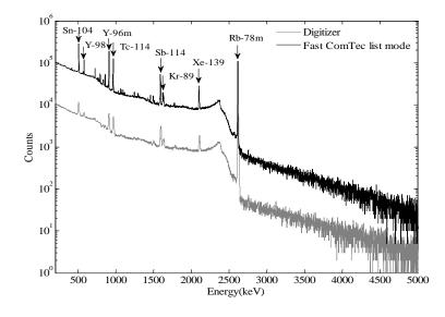
Figure 3.12 Time (>10ms) integrated delayed-fission  $\gamma$ -ray spectra from the <sup>232</sup>Th sample measured with a Fast ComTec list mode system and a customized spectroscopy system.
