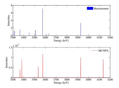
Figure 6.23 Comparison between the delayed  $\gamma$ -ray spectra published by P. Sibczynski et al. and simulation results (3.3-4.2 MeV, HEU).
