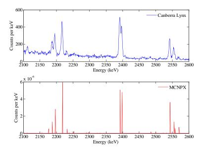
Figure 6.8 Comparison between the delayed  $\gamma$ -ray spectra measured using the list-mode system and simulation results (2.1-2.6 MeV, <sup>238</sup>U).
