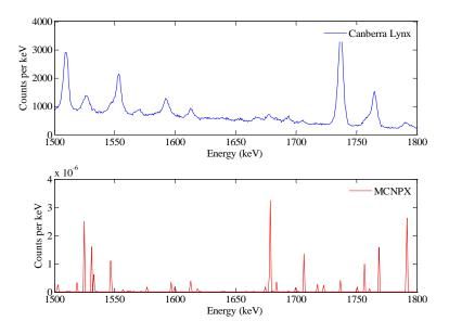
Figure 6.6 Comparison between the delayed  $\gamma$ -ray spectra measured using the list-mode system and simulation results (1.5-1.8 MeV, <sup>238</sup>U).
