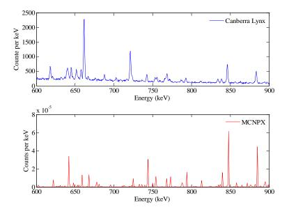
Figure 6.12 Comparison between the delayed  $\gamma$ -ray spectra measured using the list-mode system and simulation results (0.6-0.9 MeV, <sup>239</sup>Pu).
