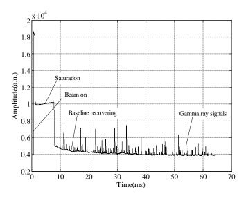
Figure 3.9 The output signal from an HPGe detector between two successive pulses.
