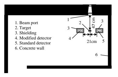
Figure 4.4 A schematic drawing of the experimental setup for testing of the effect of feedback resistor on saturation time.
