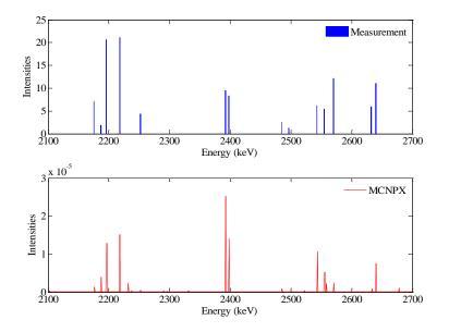
Figure 6.21 Comparison between the delayed  $\gamma$ -ray spectra published by P. Sibczynski et al. and simulation results (2.1-2.7 MeV, HEU).
