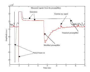
Figure 4.5 Measured signals from the preamplifiers in the photofission environment.
