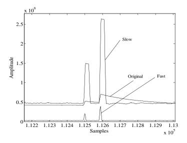
Figure 3.3 Signals from the HPGe detector; the original, fast-, and slow-channel signals are shown.
