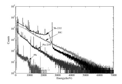
Figure 3.13 Time integrated delayed-fission  $\gamma$ -rays from various samples measured with a Fast ComTec list mode system (Note: data from the first 10 ms after each linac pulse was disregarded).
