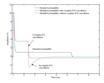
Figure 4.6 Comparison between the simulated signals from the modified preamplifier with complete and incomplete P/Z cancellations.
