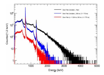
Figure 1.6 Energy spectra reconstructed using the traditional and time-variant trapezoidal filtering methods at input count rate of  $1.03 \times 10^6$  cps [1].
