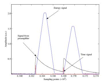
Figure 4.9 Illustration of the time and energy signal shaped in parallel in the trapezoidal filtering.
