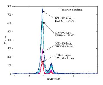
Figure 5.4 Energy spectra at different Input Count Rates (ICR) with the templatematching algorithm.
