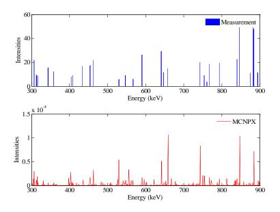
Figure 6.18 Comparison between the delayed  $\gamma$ -ray spectra published by P. Sibczynski et al. and simulation results (0.3-0.9 MeV, HEU).
