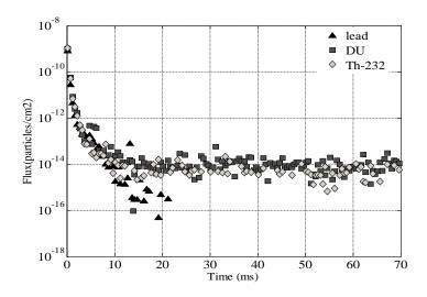
Figure 3.8 Simulated differential yields of delayed  $\gamma$ -rays from the DU, <sup>232</sup>Th, and lead samples.
