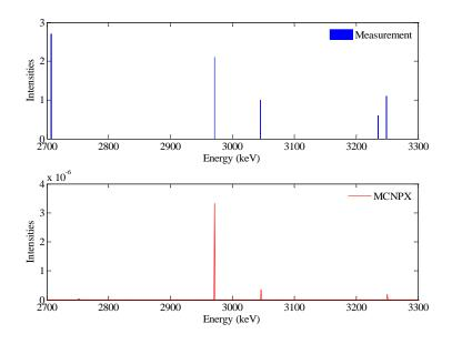
Figure 6.22 Comparison between the delayed  $\gamma$ -ray spectra published by P. Sibczynski et al. and simulation results (2.7-3.3 MeV, HEU).
