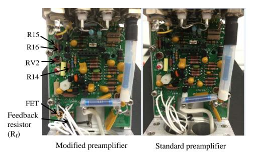
Figure 4.1 Illustration of the components of a standard preamplifier to be modified.
