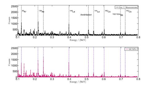
Figure 1.2 Natural uranium measurement (top) and MCNP6.1 simulation (bottom), 0.1-0.8 MeV [26].
