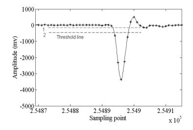
Figure 3.6 Illustration of the threshold line selection. The time width for each sample point is 10 ns.
