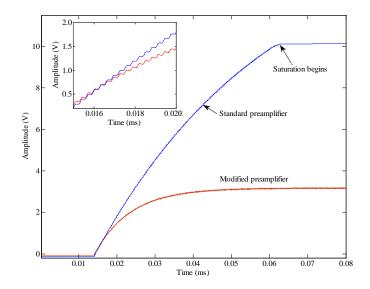
Figure 4.8 The effect of reduced tail time on baseline shift simulated in LTSpice.
