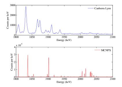
Figure 6.7 Comparison between the delayed  $\gamma$ -ray spectra measured using the list-mode system and simulation results (1.8-2.1 MeV, <sup>238</sup>U).
