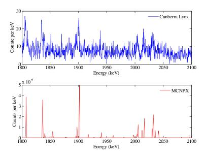
Figure 6.16 Comparison between the delayed  $\gamma$ -ray spectra measured using the list-mode system and simulation results (1.8-2.1 MeV, <sup>239</sup>Pu).
