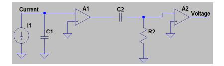
Figure 6.25 A schematic drawing of a preamplifier with RC-feedback.
