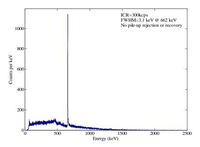
Figure 6.30 Energy spectrum reconstructed using the de-randomization method (ICR=300 kcps).
