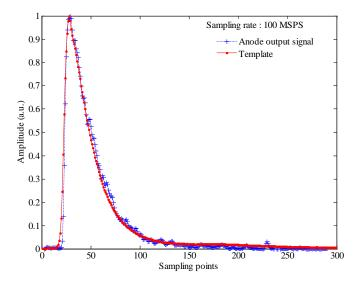
Figure 5.2 The anode output signal and the template.
