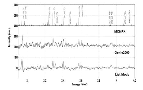
Figure 3.14 Comparison of measured and simulated delayed-fission  $\gamma$ -ray spectra above 3 MeV for DU sample.
