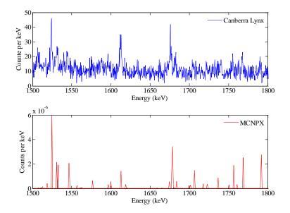
Figure 6.15 Comparison between the delayed  $\gamma$ -ray spectra measured using the list-mode system and simulation results (1.5-1.8 MeV, <sup>239</sup>Pu).
