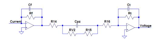
Figure 4.3 A schematic drawing of a preamplifier with RC-feedback.
