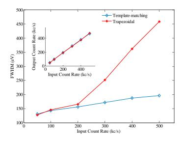
Figure 5.6 Comparison between the template-matching algorithm and the trapezoidal filter (FWHM vs Input Count Rate).
