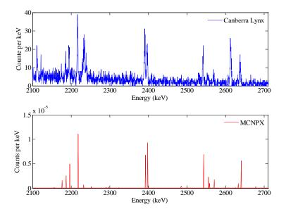
Figure 6.17 Comparison between the delayed  $\gamma$ -ray spectra measured using the list-mode system and simulation results (2.1-2.7 MeV, <sup>239</sup>Pu).
