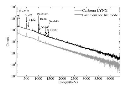
Figure 3.10 Time (>10ms) integrated delayed-fission  $\gamma$ -ray spectra from the DU sample measured with a Canberra LYNX system and a Fast ComTec list mode system.
