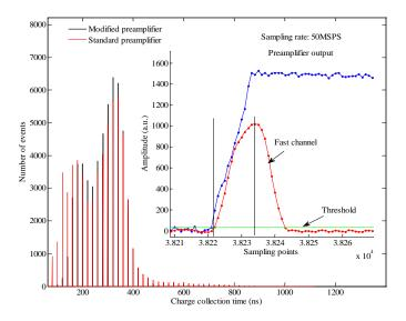
Figure 4.10 Distribution of charge collection time at input count rate of 20 kcps.
