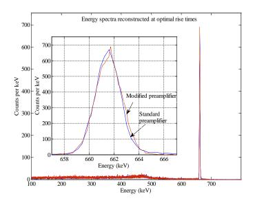
Figure 4.12 Energy spectra reconstructed at optimal rise times (flat top time was fixed at  $0.8 \ \mu$ s).
