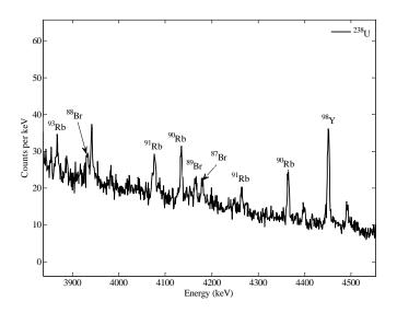
Figure 2.4 Measured high-energy delayed  $\gamma$ -rays from photofission of <sup>238</sup>U (3.9-4.5 MeV).
