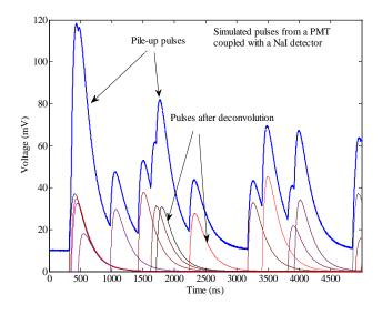
Figure 5.1 The application of the template-matching algorithm to recover simulated piled-up pulses.
