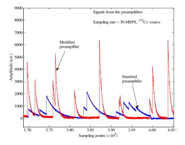
Figure 4.7 Comparison between signal waveforms measured with NI PXIe-5122.
