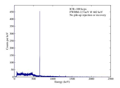
Figure 6.29 Energy spectrum reconstructed using the algorithm based on the derandomization method (ICR=100 kcps).
