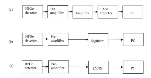
Figure 3.2 The block diagrams of the three data-acquisition systems (a. FAST ComTec list mode system; b. Customized system; c. Canberra LYNX multi-channel analyzer).
