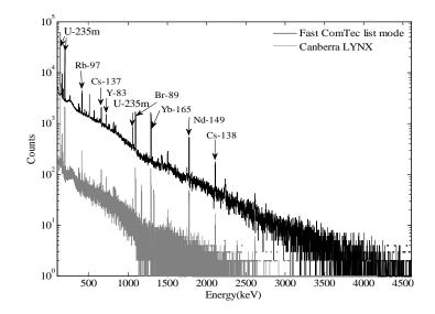
Figure 3.11 Time (>20ms) integrated delayed-fission  $\gamma$ -ray spectra from the <sup>239</sup>Pu sample measured with a Canberra LYNX system and a Fast ComTec list mode system.
