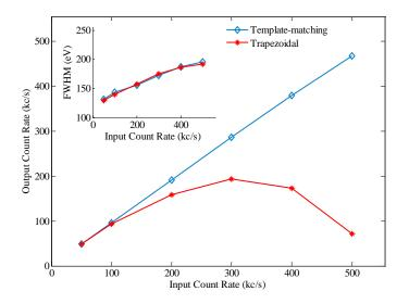
Figure 5.5 Comparison between the template-matching algorithm and the trapezoidal filter (Output Count Rate vs Input Count Rate).
