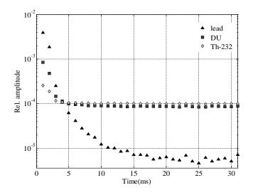
Figure 3.7 The differential yields of delayed  $\gamma$ -rays for DU, <sup>232</sup>Th, and lead.
