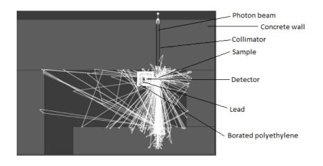
Figure 3.5 The model of the MCNPX simulation.
