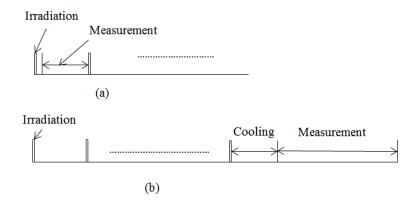
Figure 2.3 (a) Measurement of delayed γ-rays from photofission of <sup>238</sup>U in between linac pulses; (b) Measurement of delayed γ-rays from photofission of <sup>238</sup>U and <sup>239</sup>Pu after irradiation.
