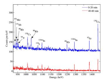
Figure 2.5 Measured delayed  $\gamma$ -rays from photofission of <sup>239</sup>Pu using the list-mode system (0.9-1.5 MeV).
