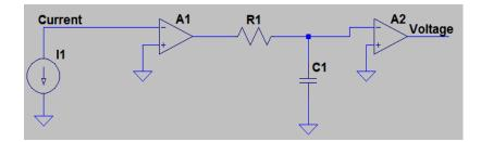
Figure 6.26 An equivalent presentation of the preamplifier.
