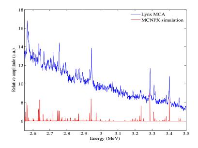
Figure 6.1 Comparison between the measured delayed gamma spectra and simulated results (2.6-3.5 MeV, <sup>238</sup>U).
