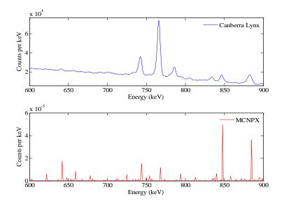
Figure 6.3 Comparison between the delayed  $\gamma$ -ray spectra measured using the list-mode system and simulation results (0.6-0.9 MeV, <sup>238</sup>U).
