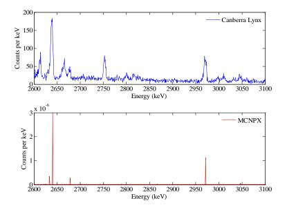
Figure 6.9 Comparison between the delayed  $\gamma$ -ray spectra measured using the list-mode system and simulation results (2.6-3.1 MeV, <sup>238</sup>U).
