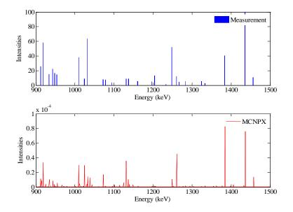
Figure 6.19 Comparison between the delayed  $\gamma$ -ray spectra published by P. Sibczynski et al. and simulation results (0.9-1.5 MeV, HEU).
