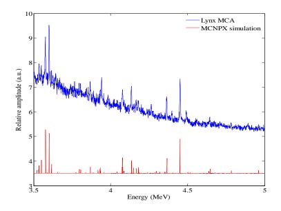
Figure 6.2 Comparison between the measured delayed gamma spectra and simulated results (3.5-5.0 MeV, <sup>238</sup>U).
