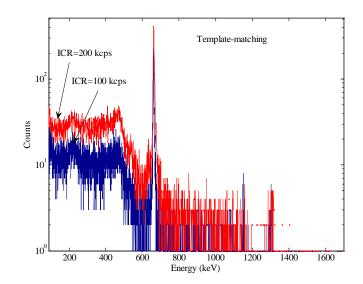
Figure 5.8 Energy spectra reconstructed with the template-matching algorithm.
