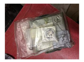
Figure 2.2 The uranium and plutonium samples used in the photofission experiments.
