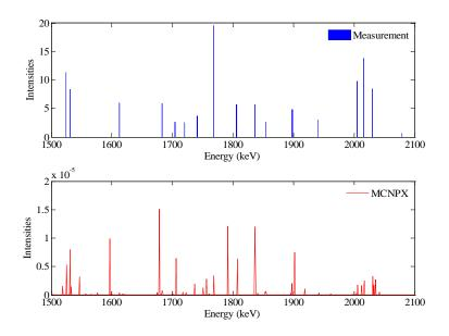
Figure 6.20 Comparison between the delayed  $\gamma$ -ray spectra published by P. Sibczynski et al. and simulation results (1.5-2.1 MeV, HEU).
