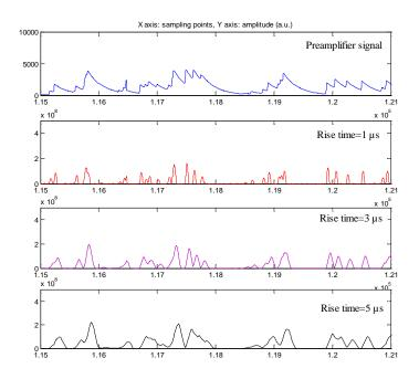
Figure 1.5 Trapezoidal filtering using different rise times (ICR=300 kcps).
