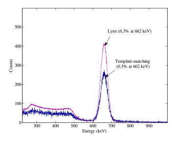
Figure 5.3 Comparison between energy spectra measured with a Canberra Lynx system and reconstructed with the template-matching algorithm.
