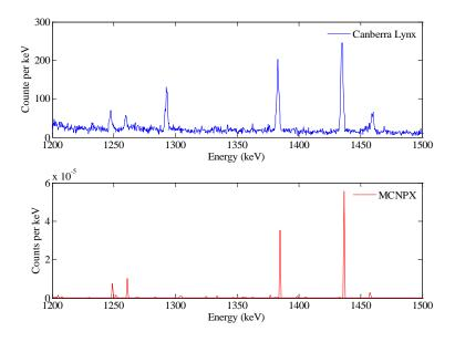
Figure 6.14 Comparison between the delayed  $\gamma$ -ray spectra measured using the list-mode system and simulation results (1.2-1.5 MeV, <sup>239</sup>Pu).
