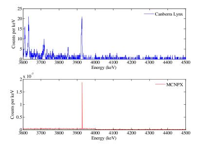
Figure 6.11 Comparison between the delayed  $\gamma$ -ray spectra measured using the list-mode system and simulation results (3.6-4.5 MeV, <sup>238</sup>U).
