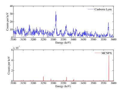
Figure 6.10 Comparison between the delayed  $\gamma$ -ray spectra measured using the list-mode system and simulation results (3.1-3.6 MeV, <sup>238</sup>U).
