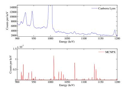
Figure 6.4 Comparison between the delayed  $\gamma$ -ray spectra measured using the list-mode system and simulation results (0.9-1.2 MeV, <sup>238</sup>U).
