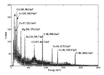
Figure 3.4 Comparison of measured spectra using the customized spectroscopy system (dots) and the commercial MCA (solid line).
