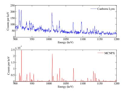
Figure 6.13 Comparison between the delayed  $\gamma$ -ray spectra measured using the list-mode system and simulation results (0.9-1.2 MeV, <sup>239</sup>Pu).
