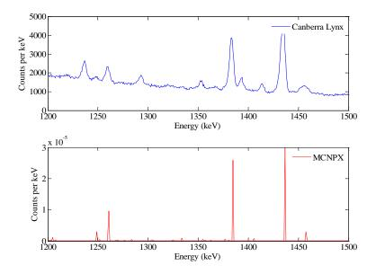
Figure 6.5 Comparison between the delayed  $\gamma$ -ray spectra measured using the list-mode system and simulation results (1.2-1.5 MeV, <sup>238</sup>U).
