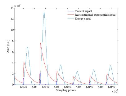
Figure 6.28 Digital synthesis of exponential pulses from the detector current signals.
