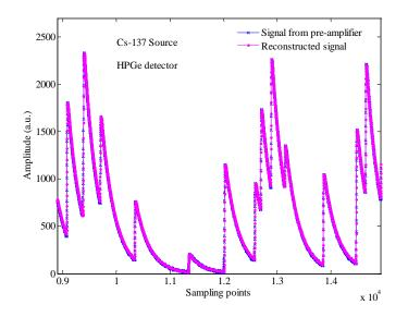
Figure 5.7 Verification of the reconstructed signal from preamplifier.
