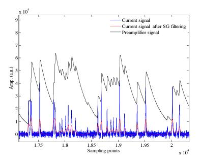
Figure 6.27 The deconvolution of pulses from an HPGe preamplifier.
