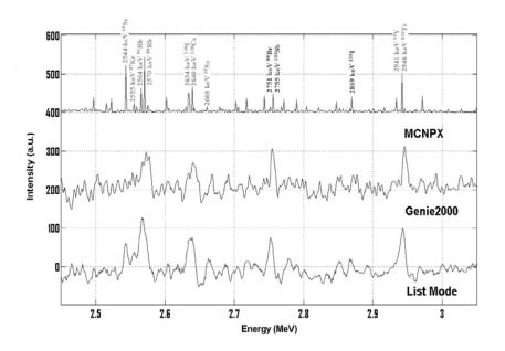
Figure 3.15 Comparison of measured and simulated delayed-fission  $\gamma$ -ray spectra from 2.5 MeV to 3 MeV for DU sample.
