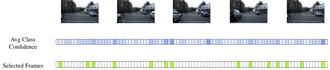
Figure 6.2: An example trajectory of running our learn budget-aware policy on a sample video from CamVid. The top row shows frames 5090 to 05180 from ‘0016E5’ video. The second row shows the color coded average confidence score for each frame where the darker means higher confidence. The third row shows the selected frames by our policy \pi . The policy is trained for B = 0.25B_{\max} using Bayesian SegNet f = [73] .
