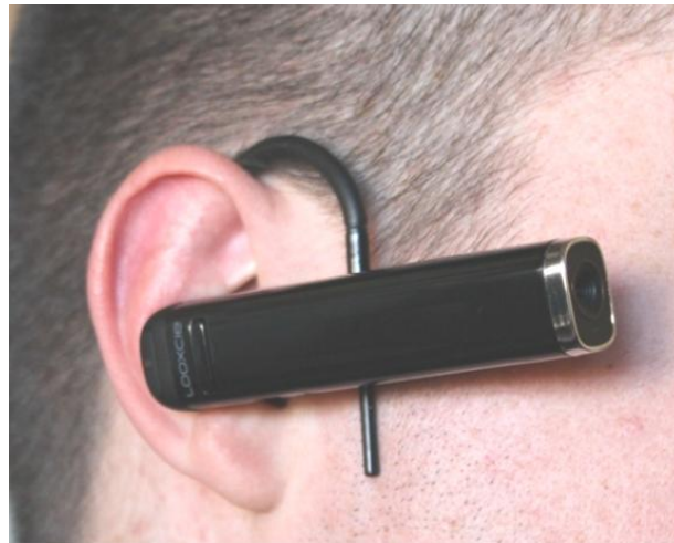
Figure 4: Looxcie Headset Camera. The “Looxcie” Bluetooth wearable headset camera was used for capturing the visitor-eye-view of interactions with docents.
