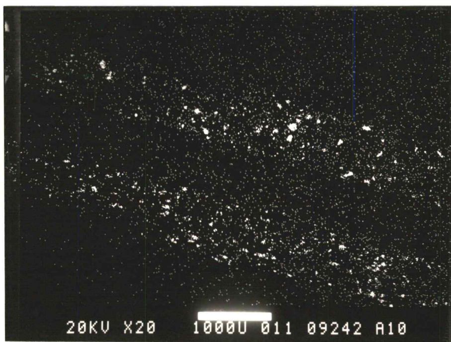
Figure 9.2 Element maps of nickel on particle surfaces for three different concentrations.
