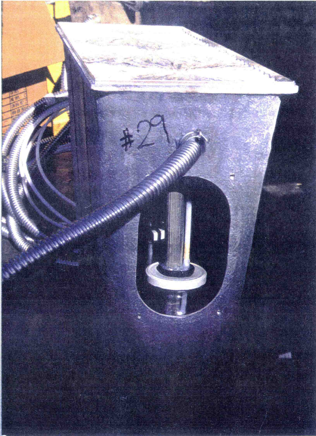
Figure 6. Passive Capillary Wick Sampler (PCAPS).
