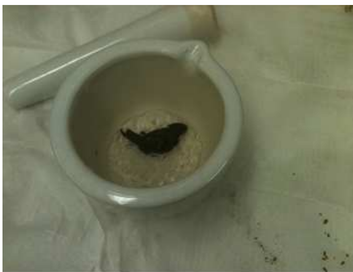
Figure 3.4 Homogenization of Animal Samples Using Liquid Nitrogen
