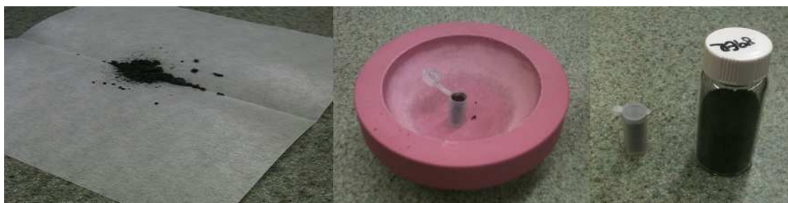
Figure 3.5 Sample and weighing paper for transfer (Left) Prevention of sample during transference (Center) Liquid Scintillation Vial and filled sample vial (Right)
