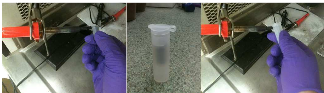
Figure 3.6 Sealing of sample vial (Left) Sample vial inside secondary containment vial (Center) Sealing of containment vial (Right)
