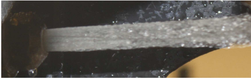
Fig. 5.9. A good-quality jet from a well-made machined brass nozzle.
