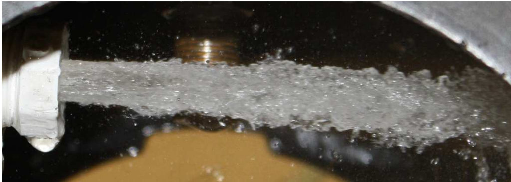
Fig. 5.10. A poor-quality jet from a homemade plastic nozzle.
