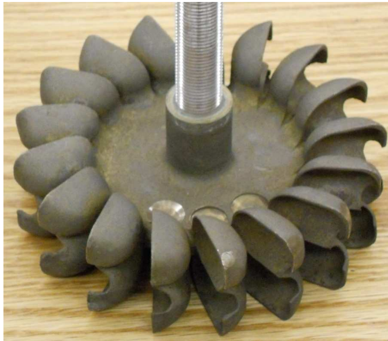
Fig. 4.3. Picture of the 100-mm Harris Pelton turbine used in this study.
