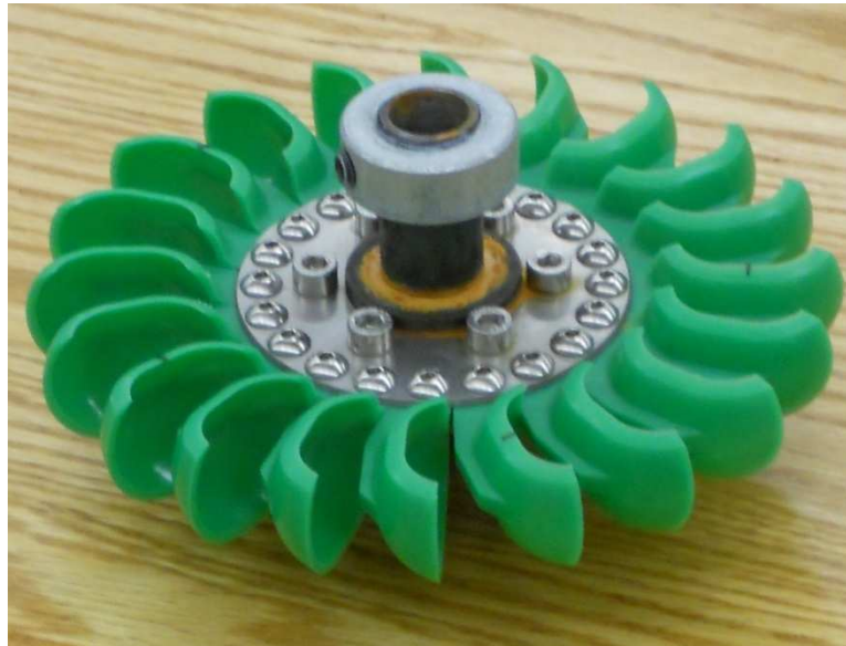
Fig. 4.4. Picture of the 133-mm Hartvigsen Hydro Turgo turbine used in this study.
