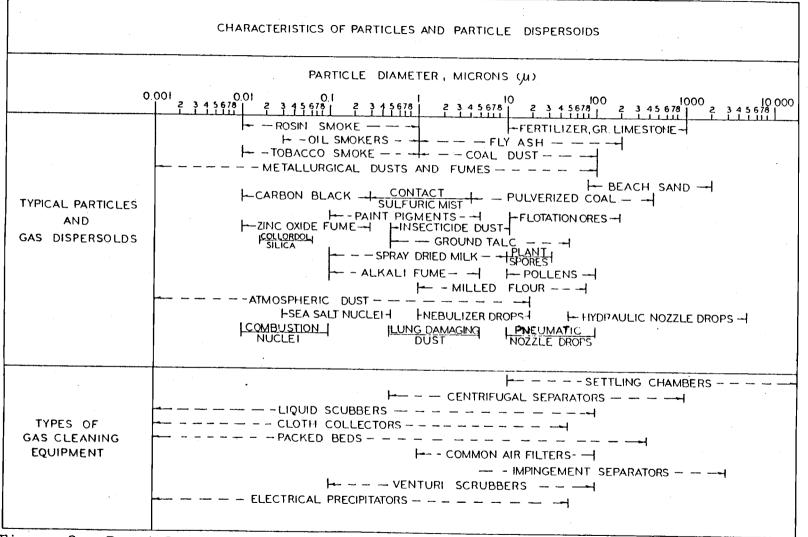
Figure 2. Particle size ranges, with typical particles and appropriate gas cleaning equipment for each range (Reference-Royco, 1973).
