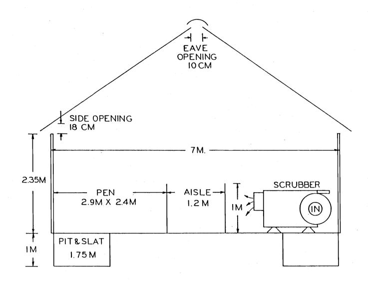
Figure 6. Cross-sectional view of the O.S.U. Swine Research Building including position of scrubber during testing.
