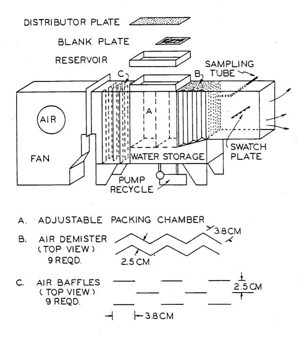
Figure 4. Diagram of cross-flow, packed scrubber used in experimentation.
