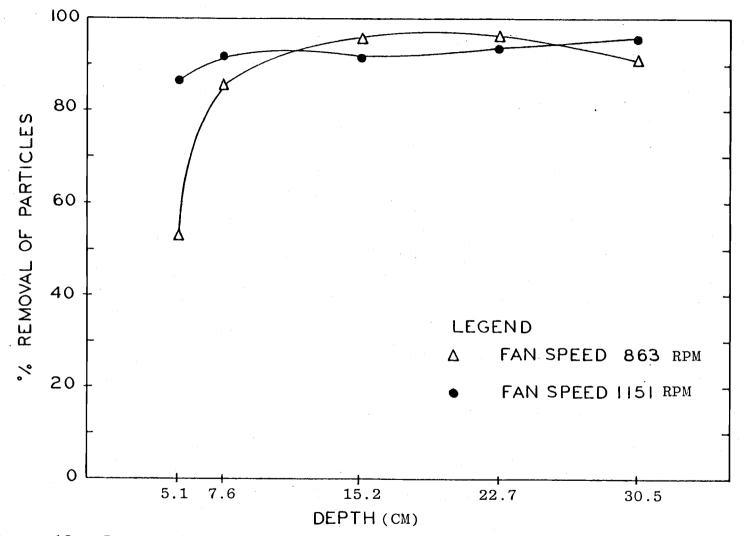
Figure 12. Interaction of fan speed and packing thickness on percent removal of  $5\mu$  particles.
