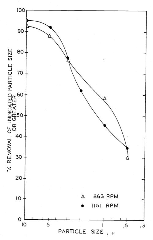
Figure 10. Percent removal of particles at two fan speeds by the cross-flow, packed scrubber,
