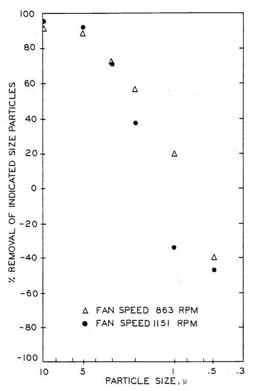
Figure 9. Percent removal of particles by a cross-flow, packed scrubber operating in a swine confinement environment.
