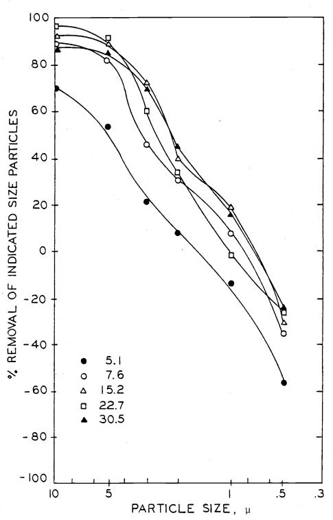
Figure 11. Percent removal of particles for five packing thicknesses by the cross-flow, packed scrubber
