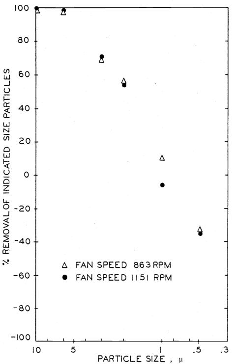
Figure 8. Percent removal of particles by cross-flow, packed scrubber in a uniform, low-dust-level atmosphere.
