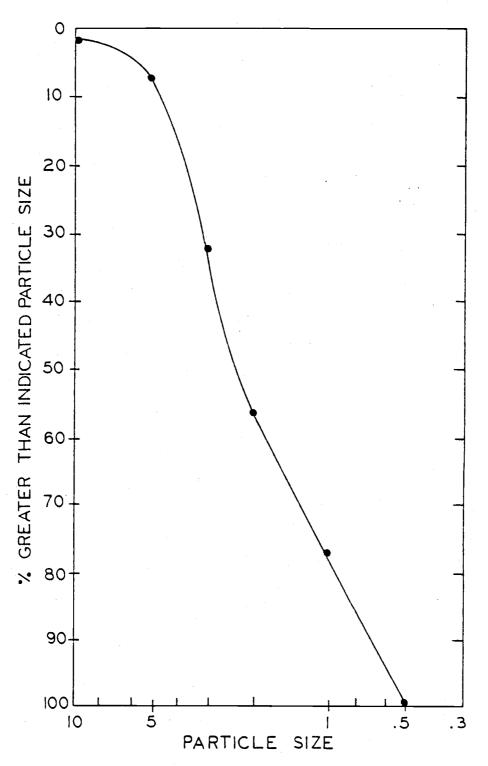
Figure 7. Size profile of the average particle load at the cross-flow, packed scrubber intake during six-week testing period at the O.S.U. Swine Center.
