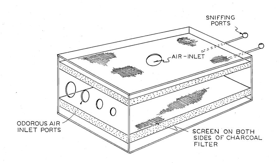
Figure 1. Diagram of the scentometer
