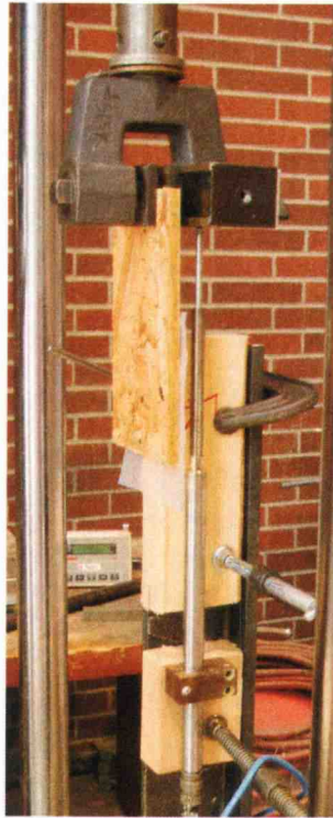
Fig. B1. Modified lateral connection test set-up.
