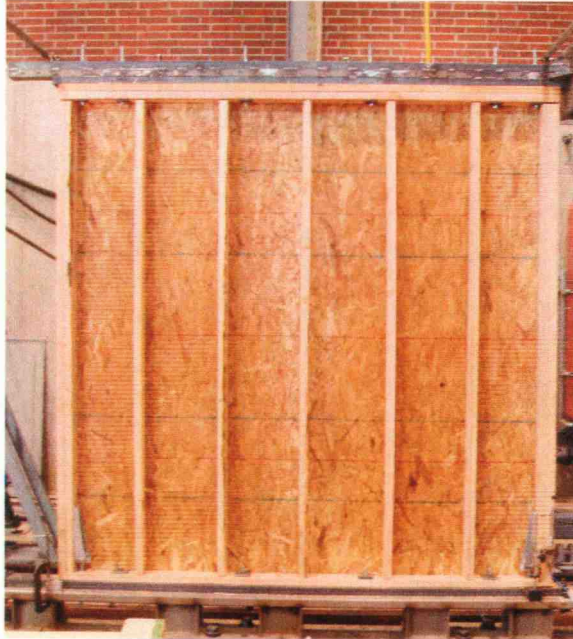
Figure C1. Shearwall test set-up.
