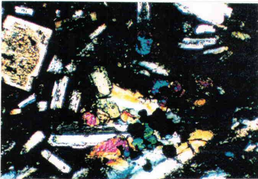
Figure 2.2 (continued). 4) Photomicrographs from the Hyalite volcanic center samples: a) Sample HGB1395 from the base of the flow sequence with a fine grained microlitic texture with small phenocrysts of augite (center), with groundmass olivine and plagioclase, and b) Sample HGB395 from the top of the sequence with plagioclase, augite and magnetite in hyaline groundmass. (Crossed polarized light for all photos; field of view = 4 mm across.)
