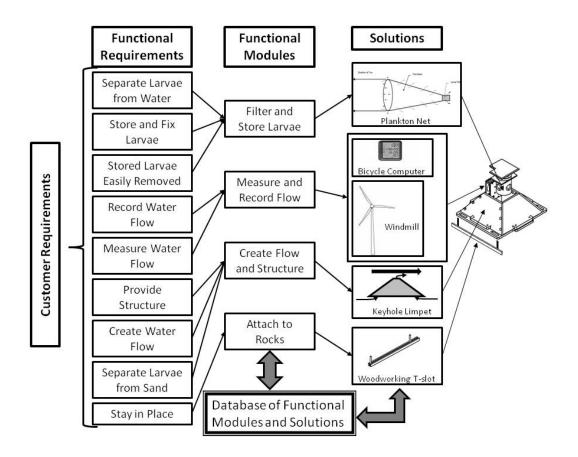
Figure 2.3. Diagram showing the design sequence for the larval collector. Customer requirements were collected and functional requirements were generated which were then grouped into functional modules. Solutions were identified for each functional module and then the interfaces between modules were modified to create the final product. A database would interact with both solutions and function modules.
