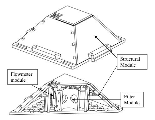
Figure 3.2. Onshore larval collector. The top view shows the collector in its entirety and the bottom view is a cross section with three of the four main modules indicated. The fourth module that attaches the collector to the rocks has been omitted.
