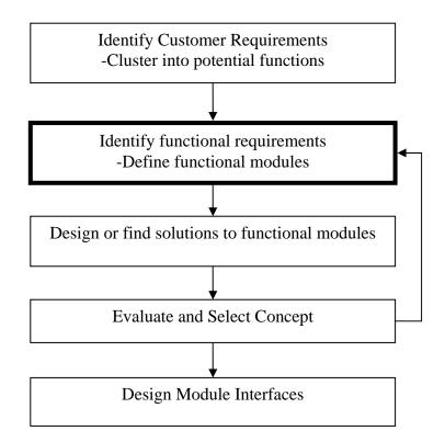
Figure 3.1. Methodology Overview: a Flow chart displaying steps for designing modularity into low production volume products. The stage outlined in bold is the primary step where modularity is incorporated.
