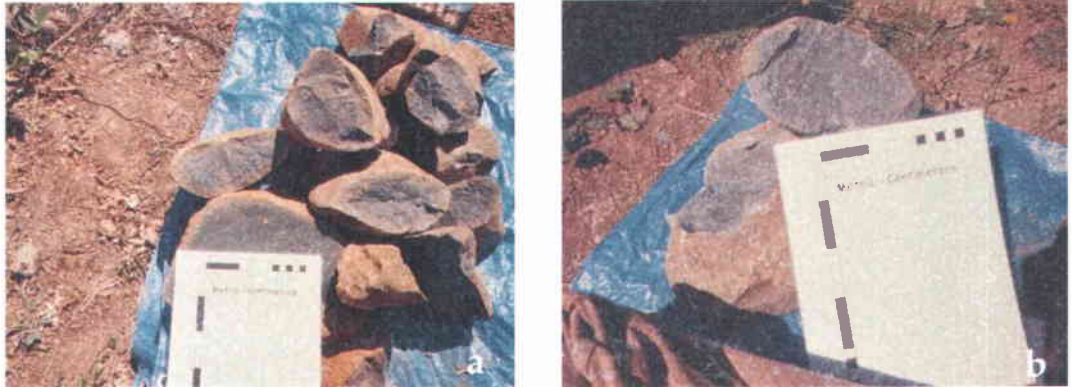
Figure 2.5 a. Weathering rinds on clasts from the Springwater geomorphic surface. b. Weathering rinds on basaltic clasts from Qt_3 the Estacada terrace.
