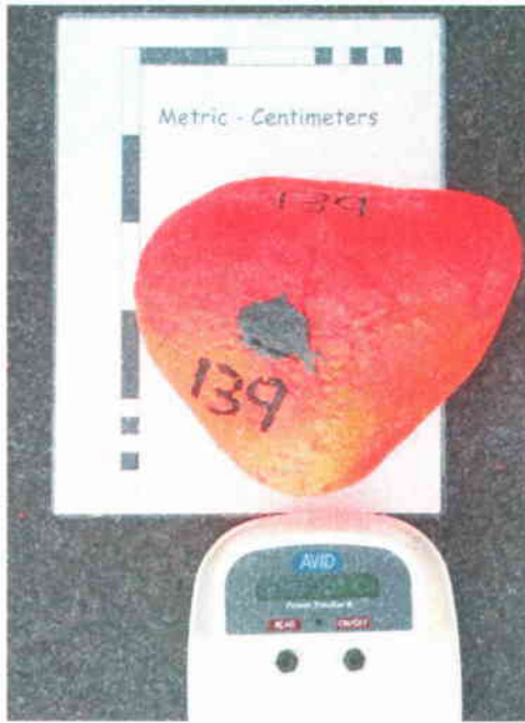
Figure 4.11 Painted tracer rock with Passive Integrated Transponder (PIT) tag reader.
