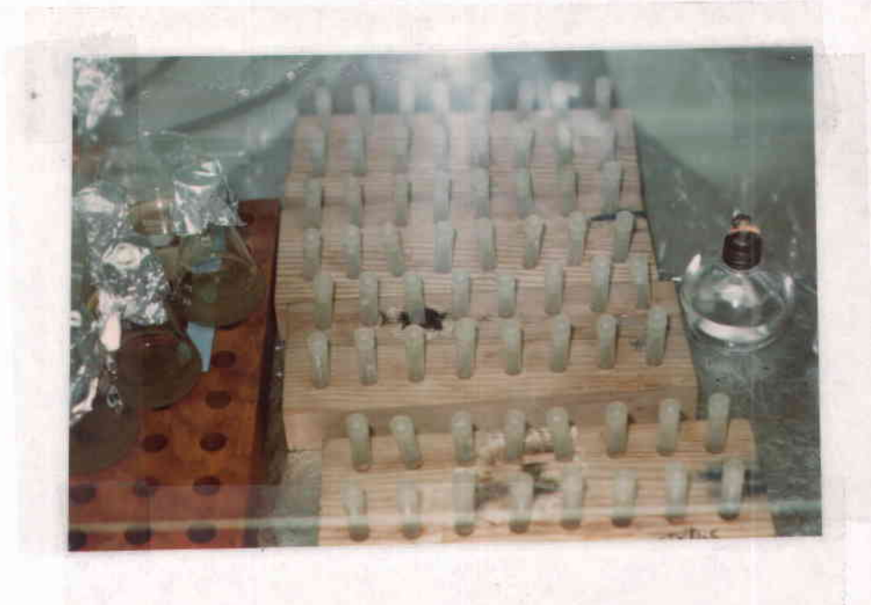
Figure 17. Cryotube ampules containing cell clumps to be frozen. Flasks on left contain test material. Aseptic conditions must be maintained.
