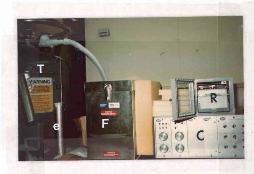
Figure 18. Freezing apparatus showing low pressure liquid nitrogen tank (T), freezing chamber (F), control unit (C), and chart recorder (R). Container to lower and hold frozen samples in liquid nitrogen storage tank is shown at "e".
