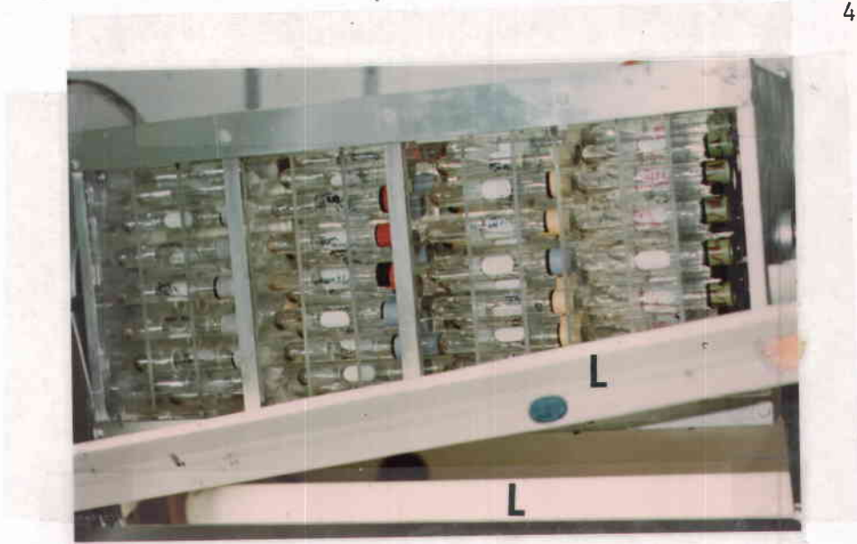
Figure 15. Rotating apparatus containing 13 x 100 mm culture tubes for treatment testing of cell cultures. Note lights at "L".
