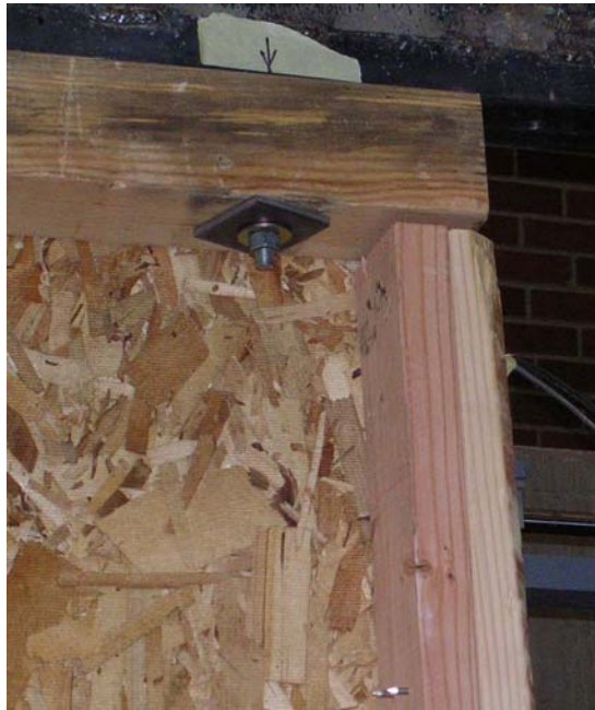
Fig. B19. Conventional shearwall top-plate separation.
