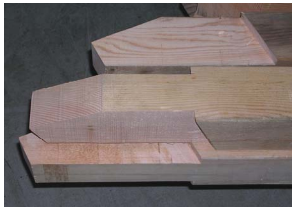
Fig. A8. Braces cut to accommodate plywood gusset plates.
