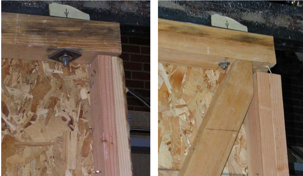
Fig. 3.7. Type 1 shearwall top-plate separation (left) and Type 2 braced shearwall top-plate separation (right).
