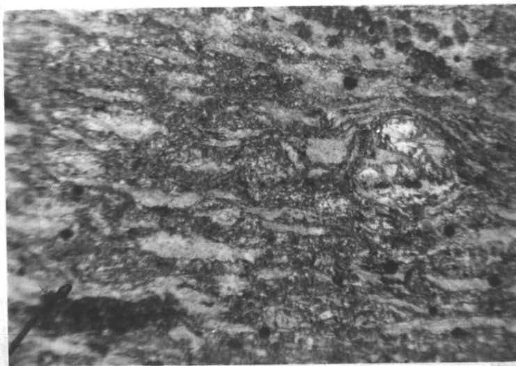
Figure 52. Photomicrograph (about X 40, plane light) of a mylonitic spilite of the Oxbow-Cuprum shear zone. Albite porphyroclast in right-center.
