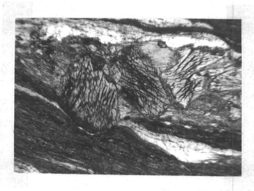
Figure 54. Photomicrograph (about X 40, plane light) of mylonite derived from a diorite of the Oxbow-Cuprum shear zone. Hornblende porphyroclasts in center of photograph.
