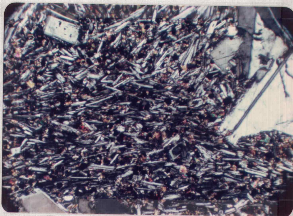
Figure 16. Pilotaxitic texture of the older basaltic unit. Crossed nicols.
