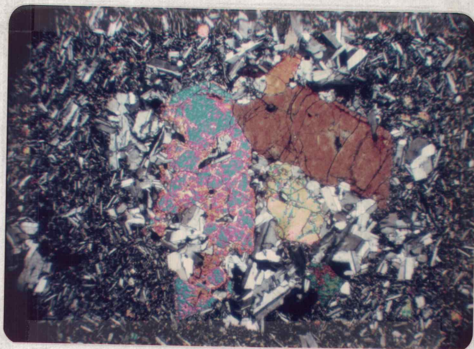
Figure 15. Glomerocryst of olivine and plagioclase in the coarse-grained member of the older basaltic unit. Crossed nicols.
