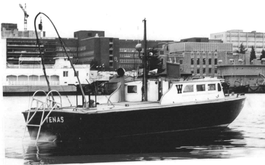
Figure 9. Research vessel Tenas . Note diving ladder, and winch to lower concrete anchors.
