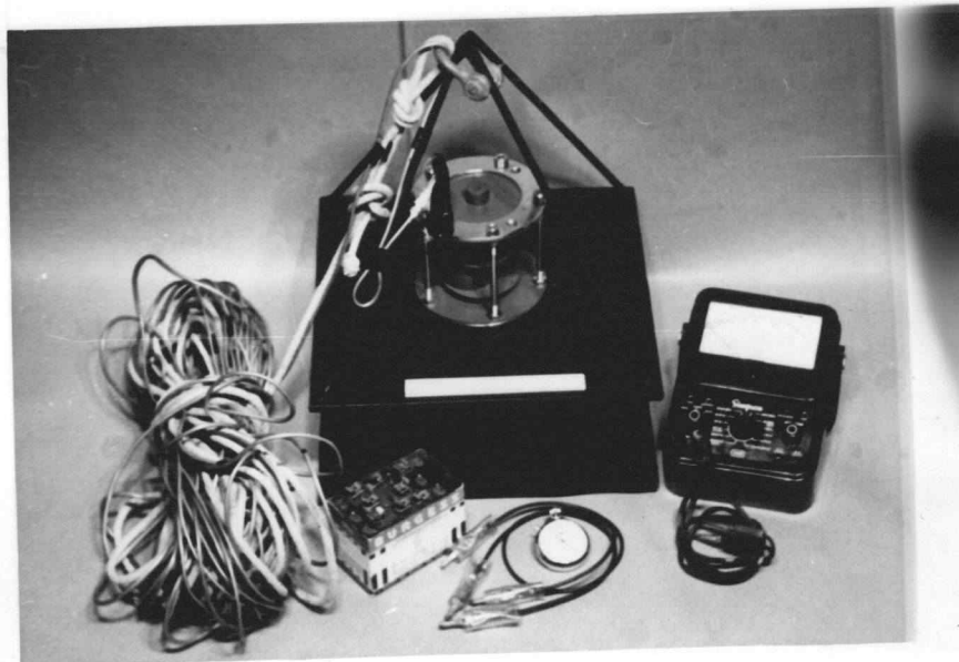
Figure 14. Current rate meter, battery, and volt-amp meter, ready for use.
