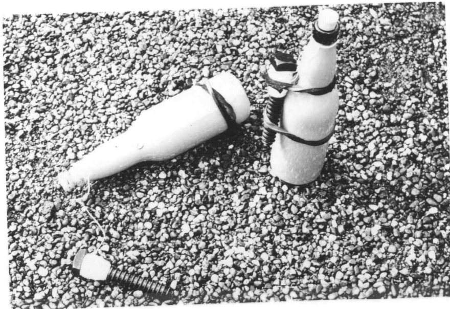
Figure 8. "Beer-bottle buoys" used to mark and map the Sludge Bed Station. Bottles floated and the bolts, which were shoved into the sediment, held the bottles in place.
