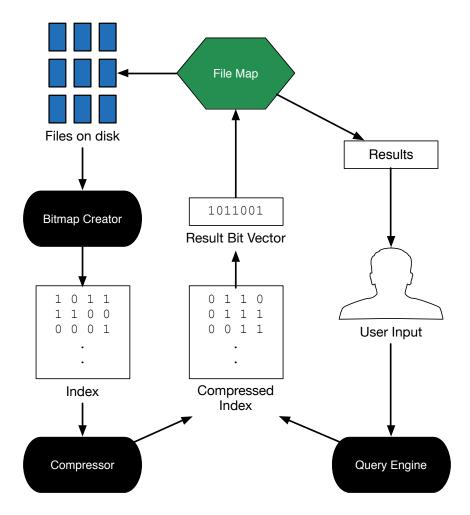
Figure 2.1: PMU Data Management System Architecture
