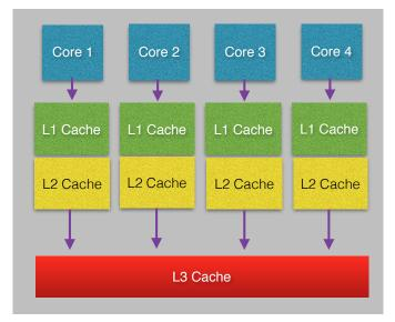
Figure 3.1: CPU cache for test implemented
