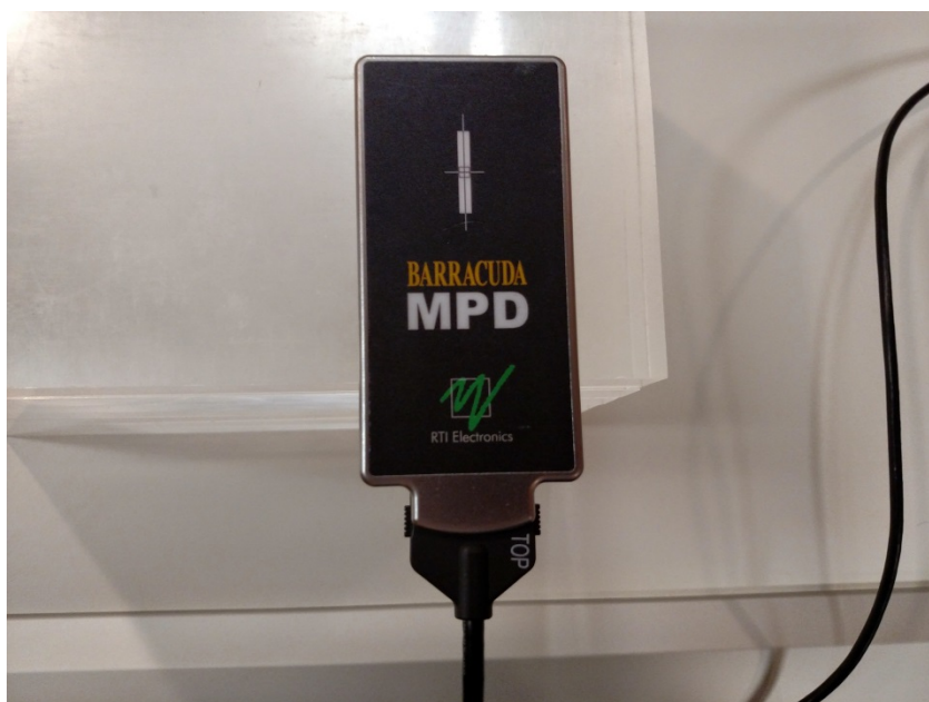
Figure 3. The RTI Multi-Purpose Detector positioned on a stack of PMMA blocks.
