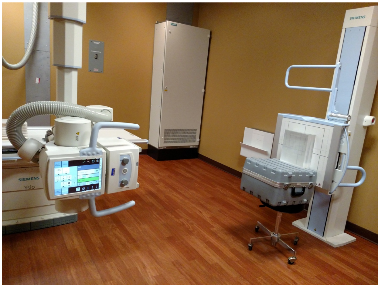
Figure 4. Radiographic tube positioned toward the upright AEC device with a PMMA phantom in the radiation field.
