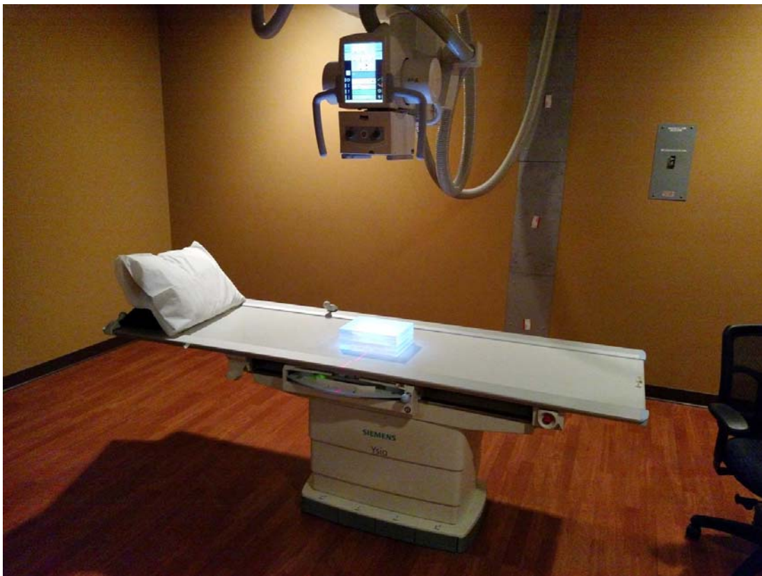
Figure 5. Radiographic tube positioned toward to the table AEC device with a PMMA phantom in the radiation field.
