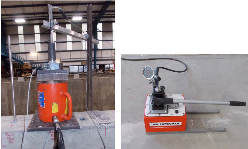
Figure 3.36 – Pullout test setup and hydraulic hand pump
