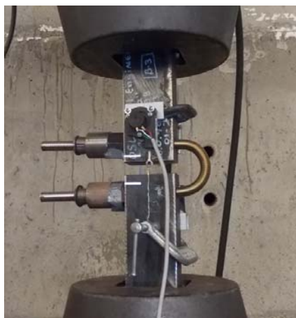
Figure 4.45 – Sample 180° hook in test setup
