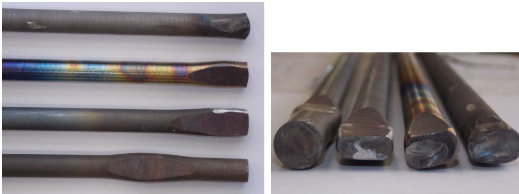
Figure 3.35 – Bulb end samples for pullout testing
