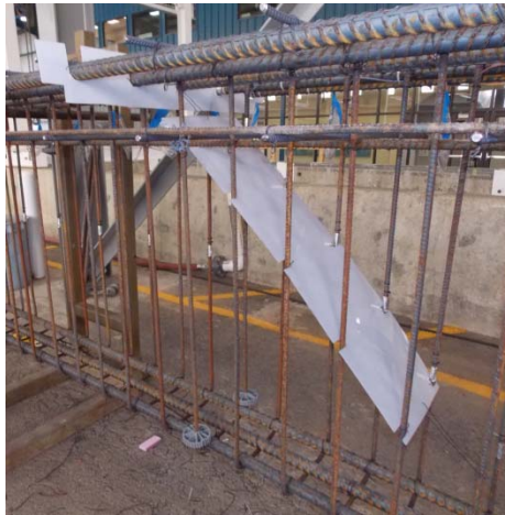
Figure 3.15 – Preformed crack placement
