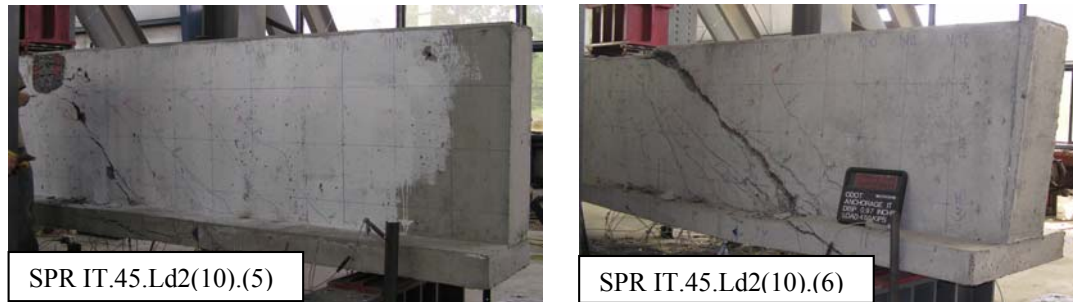
Figure 4.8 – Failure photographs of SPR test specimens
