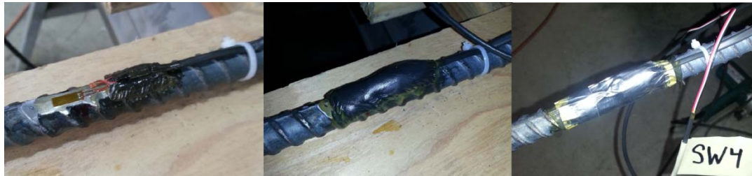
Figure 3.23 – Strain gage waterproofing and protection
