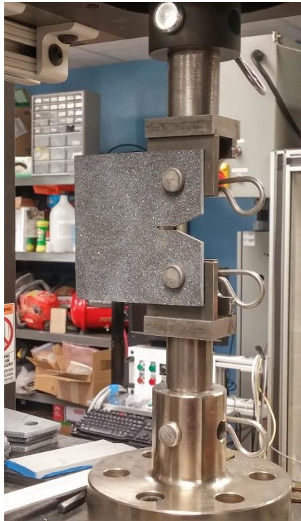
Figure 3-4: Custom pin and clevis fixture used to hold and load the specimens. The pins at the top were placed into the holes of the specimen and the bottom pins were in the load cell and load frame.
