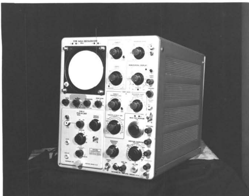
Plate 3. The Tektronix Oscilloscope (Model 545-A), type K plug-in preamplifier and P16 phosphor, cathode ray tube.
