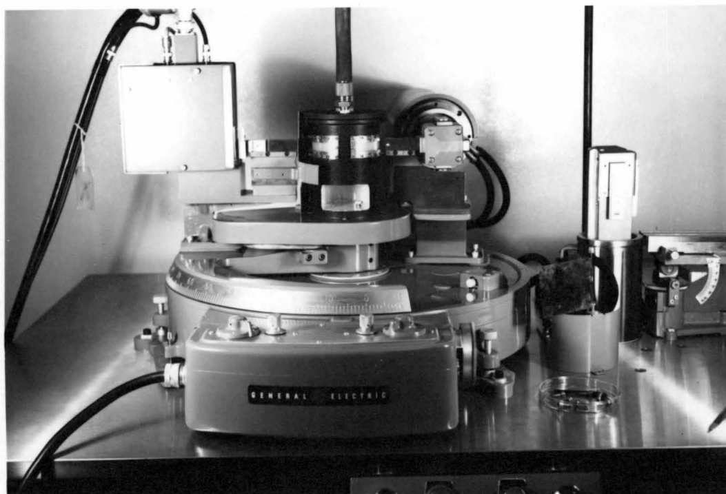
Figure III. X-ray diffraction spectrogoniometer and vacuum chamber.
