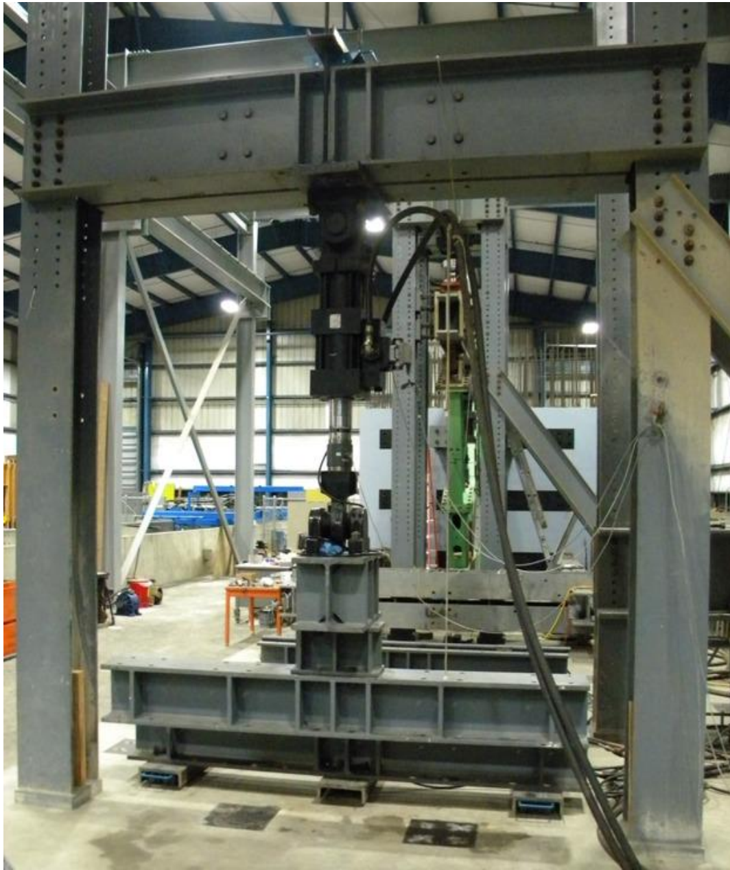
Figure 4.17: Test setup 1 for stiffness and load distribution tests
