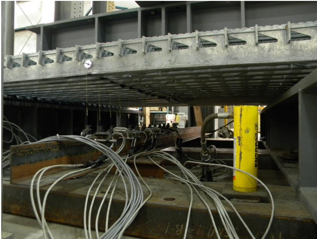
Figure 4.33: Strain gages and displacement sensors on specimen 4.0RECT2.5TYP4
