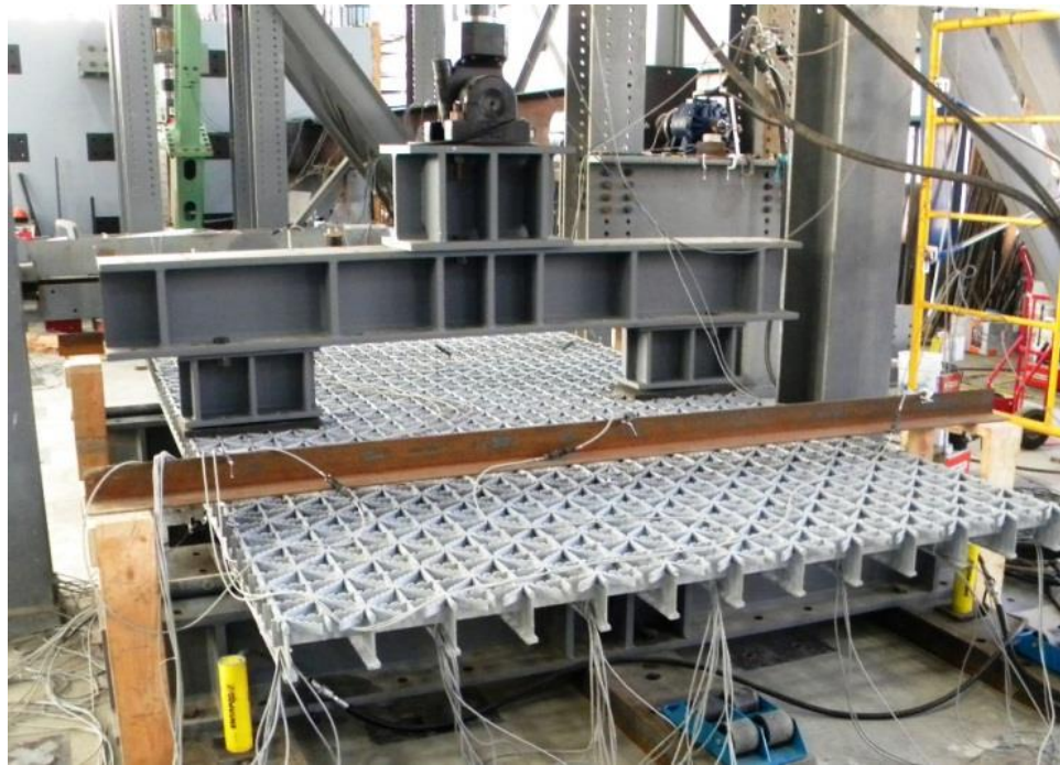
Figure 4.25: Simply supported 8 ft span with axle load parallel to main bars
