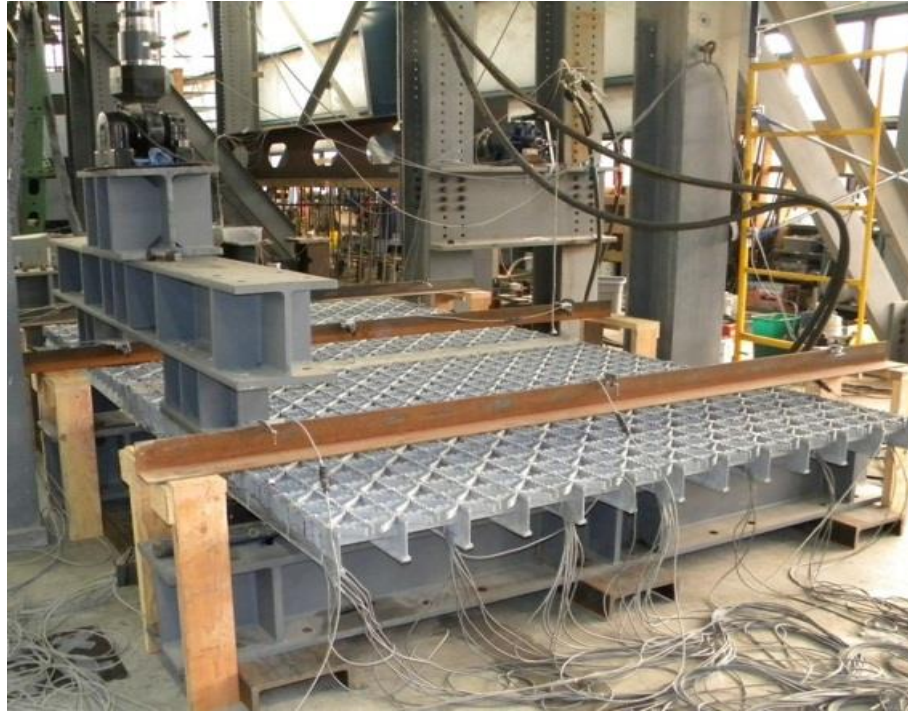
Figure 4.30: 5 ft axle, negative moment fatigue setup
