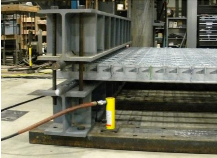
Figure 4.26: Pinned condition for far support of continuous span tests
