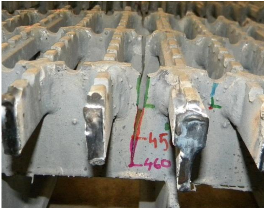
Figure 5.31: 'N' crack initiation from serration punch-out
