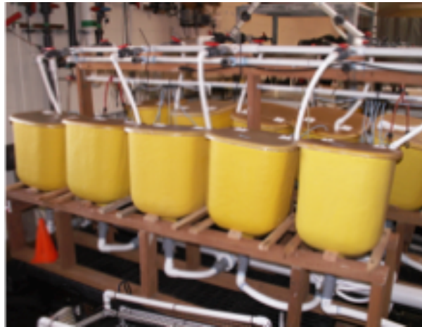
Figure 1.2. Example of a small-scale oyster depuration system. Flow-thru depuration systems at Hatfield Marine Science Center, Newport, OR. Filtered seawater, combined with algae is pumped through the lines and the effluent drained out the bottom where they are treated in accordance with quarantine procedures at HMSC.
