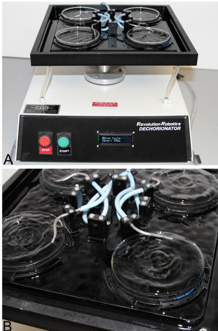
Figure B- 1. A modified shaker platform-based instrument for the automation of chorion removal from zebrafish embryos at 4 hours post fertilization.
