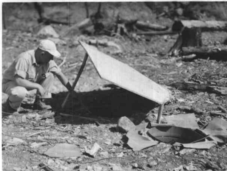
Figure 12. Close-up View of Experimental Temperature Apparatus Showing Insulated and Shaded Tubs.
