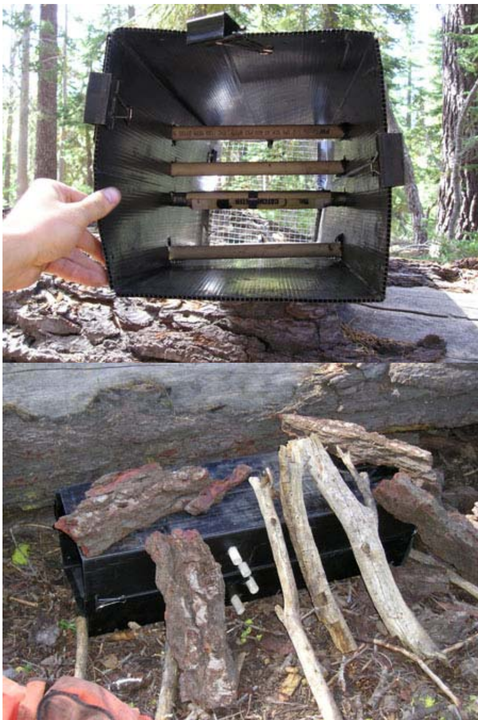
Figure A.1 3. Track plate hair snare used to detect martens in summer 2007 at Sagehen Creek Experimental Forest, CA.
