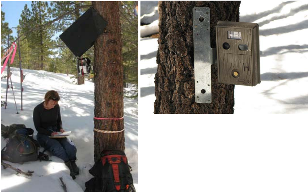
Figure A.1 5. Digital cameras (Cuddeback, model Excite) with an insulated jacket were used to detect martens at Sagehen Creek Experimental Forest, CA winter 2007–2008.
