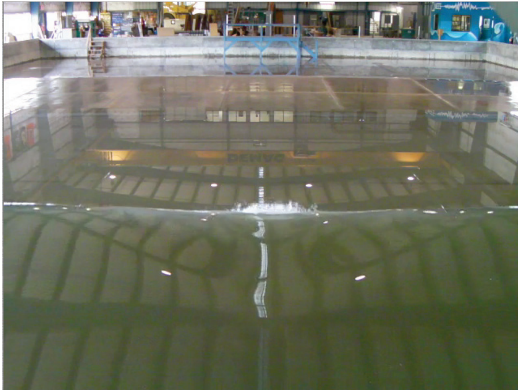
Figure 7: View of the wave propagation in the 3D wave basin at OSU; shows a breaking wave over the triangular sloping shelf
