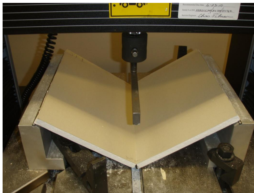
Figure B2. GWB Flexural Test Setup
